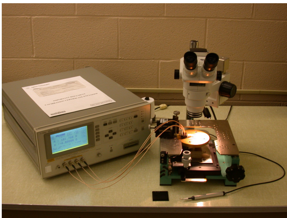
Figure D.3 – Agilent 4284A Connected to the J micro Technology JR-2727 Probe Station through Four Fifty-ohm Coaxial Cables
