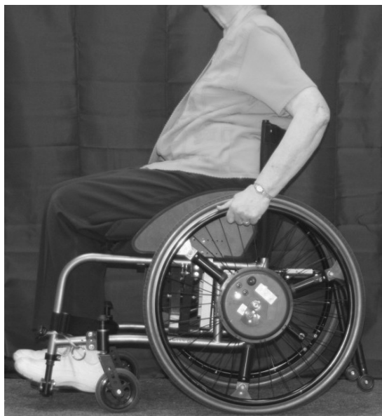
Figure 1.1 Older Adult seated in a test wheelchair with elbow angle at 100 - 120°
