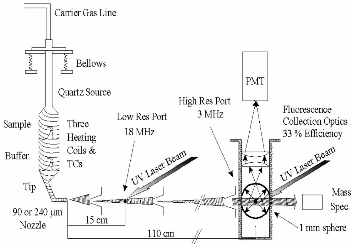
**Figure 5. Schematic diagram of the molecular source and the collection optics.**
