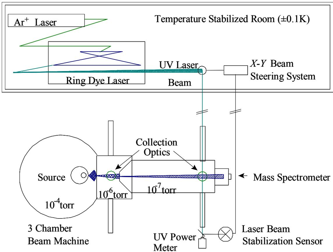
**Figure 1. Overall layout of the high resolution laser spectrometer.**
