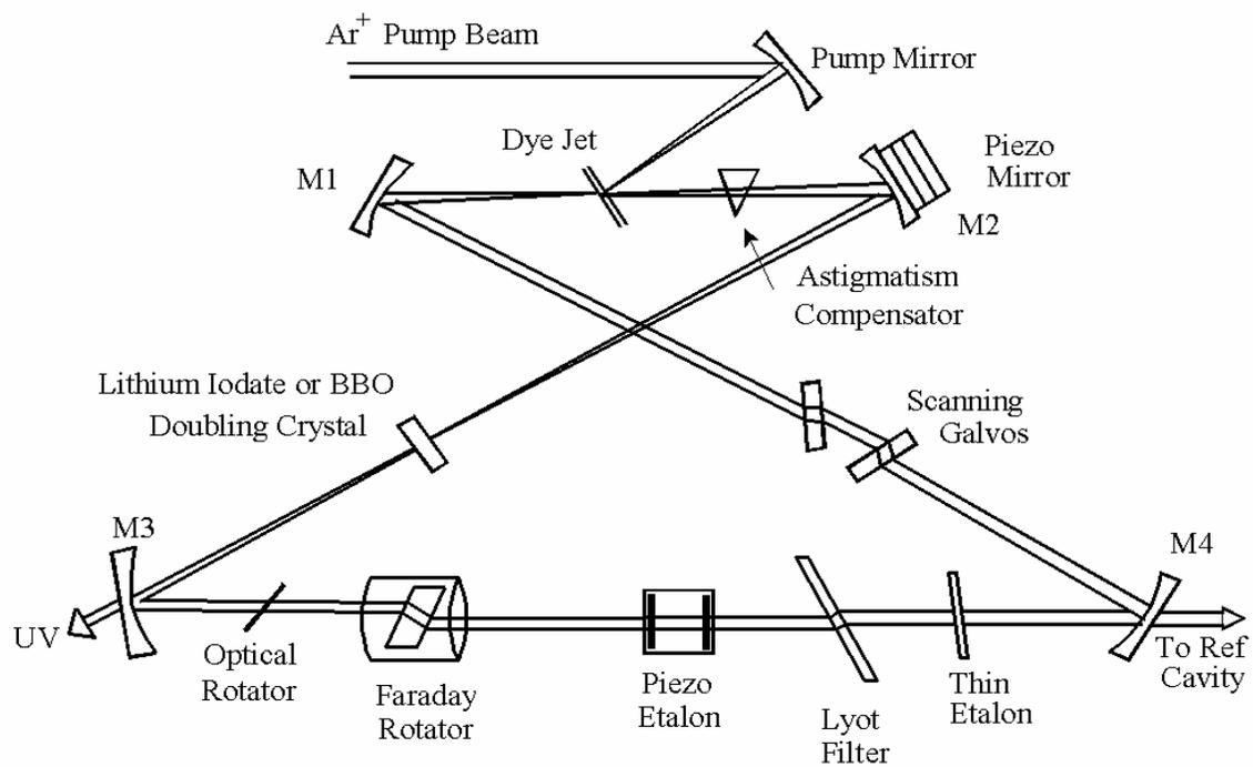
**Figure 2. Schematic diagram of the high resolution CW ring dye laser.**
