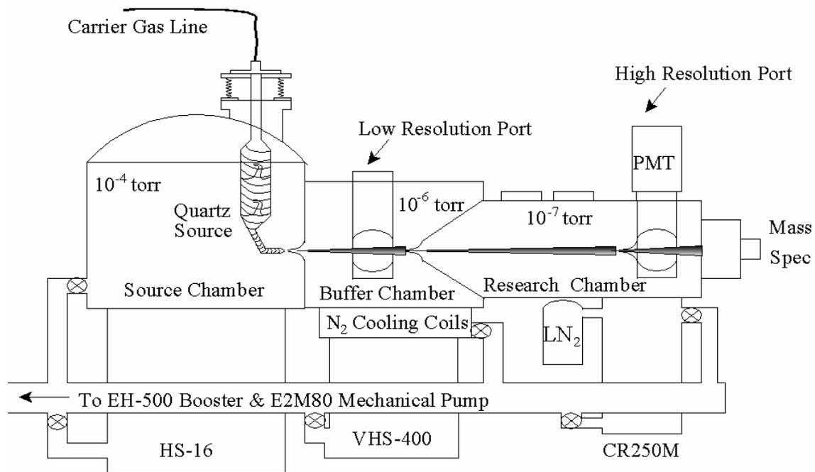
**Figure 4. Schematic diagram of the molecular beam machine.**
