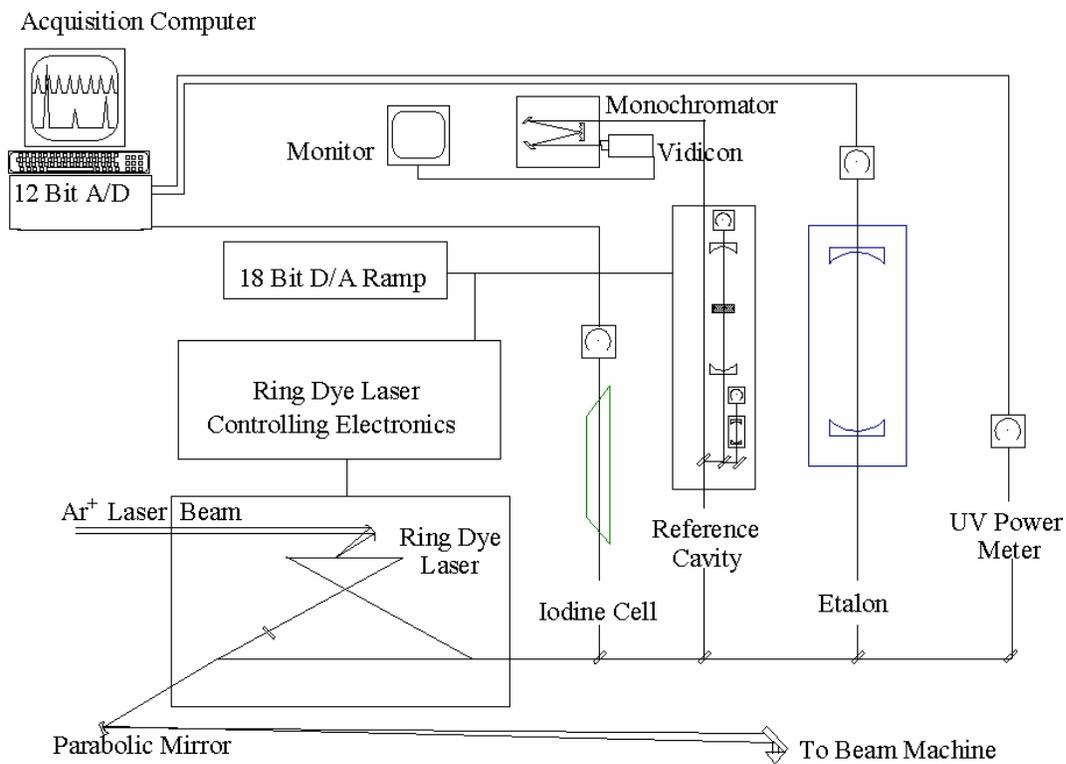
**Figure 3. Schematic diagram of the stabilization system.**
