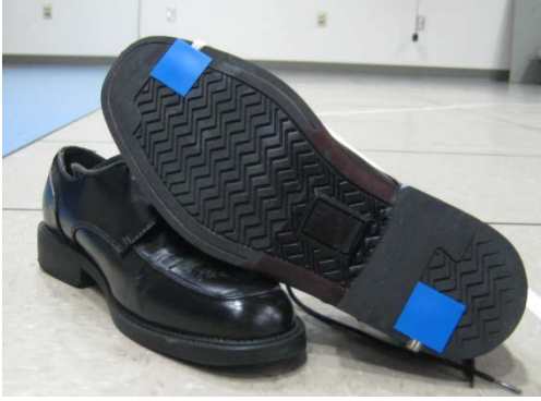
Figure 4: Polyvinyl soled shoe instrumented with two simple on-off membrane switches for temporal heel contact and toe off events.
