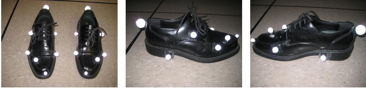
Figure 3: Anterior (left), lateral (middle), and medial (right) views of motion capture marker placement on polyvinyl soled shoes for testing. A total of nine markers were used on each foot including one on the lateral malleolus (not shown).
