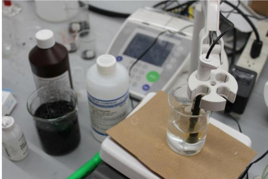
**Figure 3.11.** System used for measuring nitrate concentrations in the laboratory.
