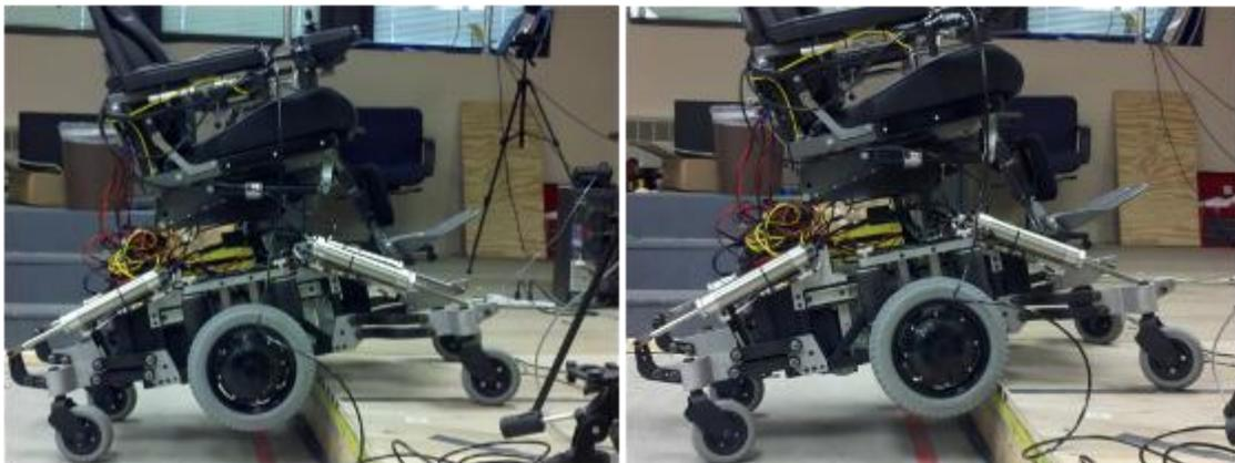
Figure 6-4: PerMMA Gen II in automatic climbing mode
