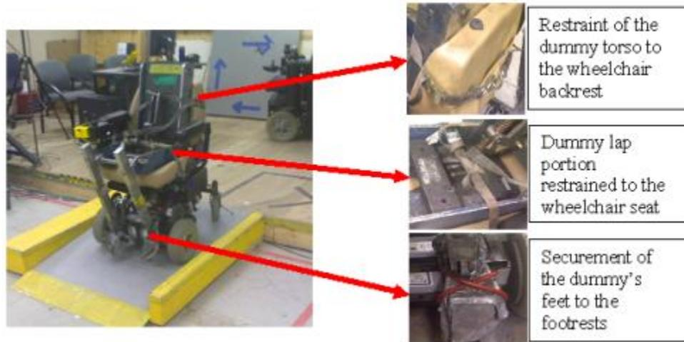
Figure 4-13: Experimental setup of the EPW
