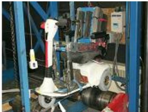
(a) A scooter set up on the DDT machine
