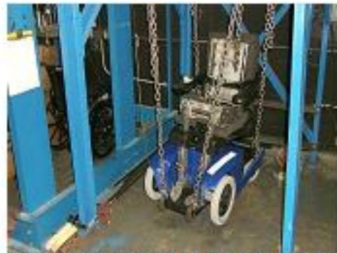
(b) A EPW set up on the CDT machine
