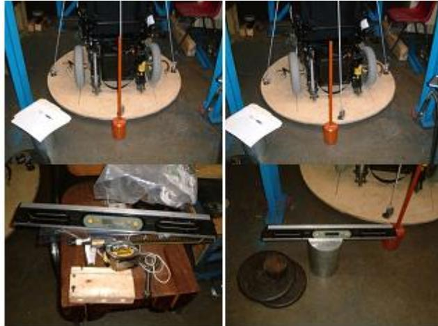
Figure 3-5: Photographs of the motion of the bottom plate with the EPW on the plate and the devices (gradienter, stopwatch, rulers, etc.) and materials (metal disks, cylinder) used in the experiment
