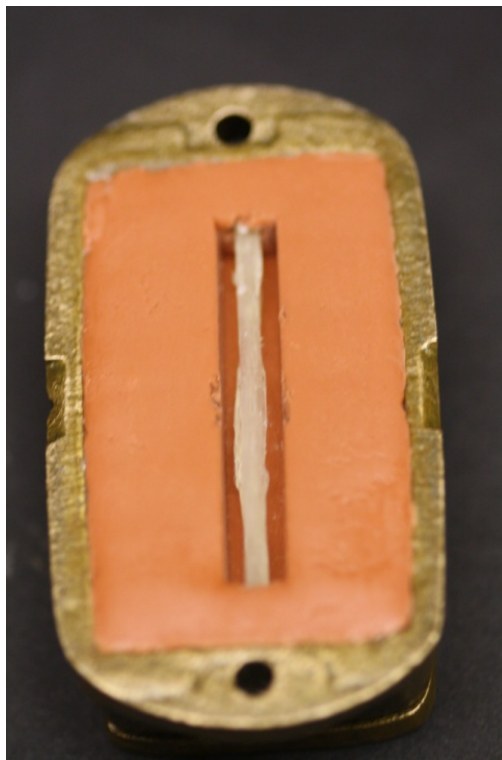
Figure 8: Impregnated glass fiber positioned within lateral slots
