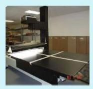
Maps are scanned on a Cruse Table Scanner CS 285/1100 ST/FA equipped with a 58" x 90" vacuum table at the
