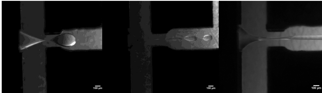
Figure 46 A: drop formation in the cross-flow junction for water. B. Formation of a short filament with downstream breakup with PEO400. C. Formation of a filament without downstream breakup. The continuous phase fluid here is PDMS 100K. P_c here is 10 psi, P_d is 4.73 psi.
