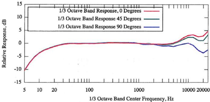
This frequency response measurement is not a NIST-traceable calibration.
