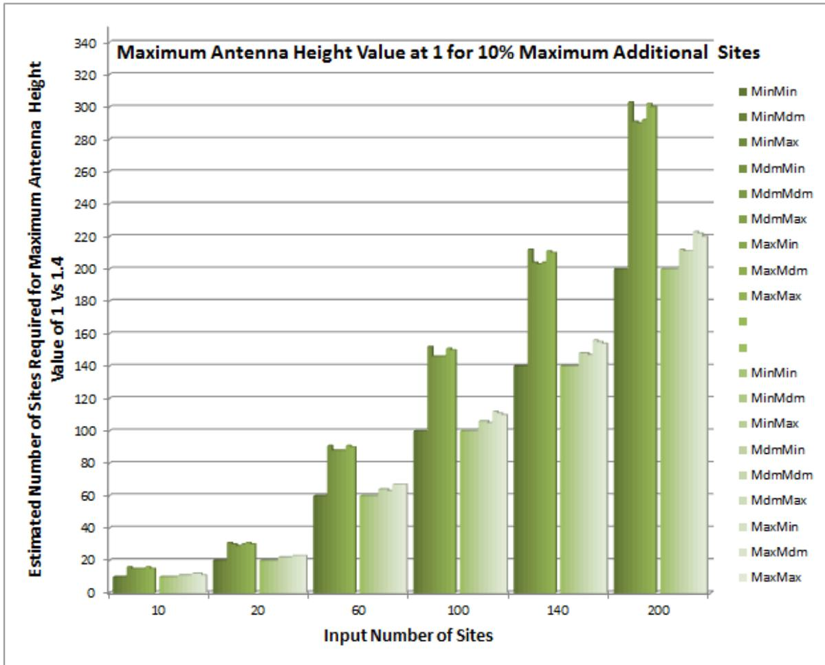
**Figure 13: Maximum antenna height set at 1 for all permutations of system configurations**
