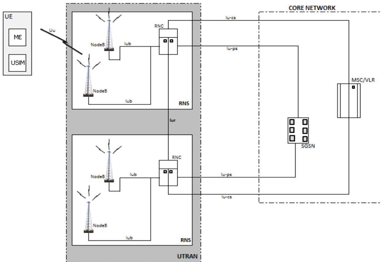
**Figure 3: The UMTS Terrestrial Radio Access Network (UTRAN) [2]**
