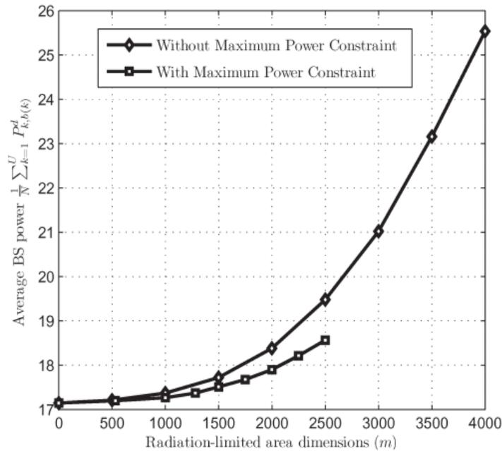
**Figure 6: Pareto-optimal set that provides the tradeoff between BS power and the dimensions of the radiation-limited area for a uniform user distribution [24]**
