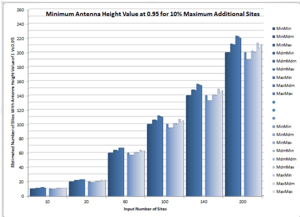
**Figure 12: Minimum antenna height set at 0.95 for all permutations of system configurations**
