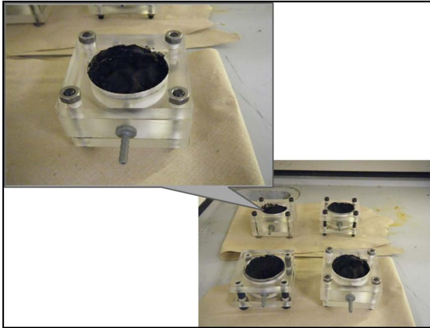
**Figure B3. Drying after application of activated carbon.**
