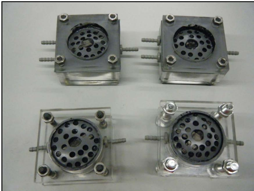
**Figure B4. Completely assembled SCMFCs, including stabilizing bolts and inlet/outlet ports.**
