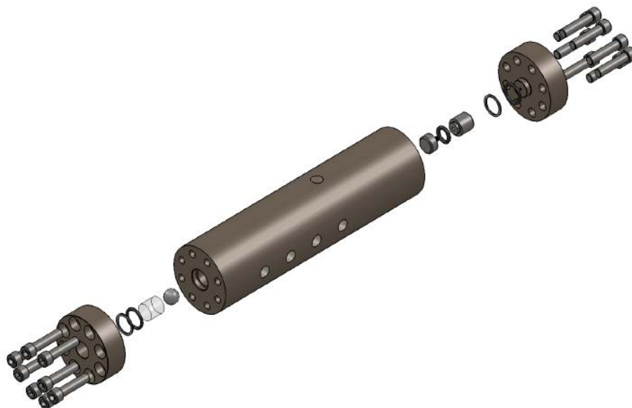
Figure 27: Expanded view of the HTHP rolling ball viscometer used in this study. The front window and rolling ball are shown on the left-hand side of the viscometer body. The floating piston that separates the test fluid from the overburden fluid (water) is shown on the right-hand side of the viscometer body
