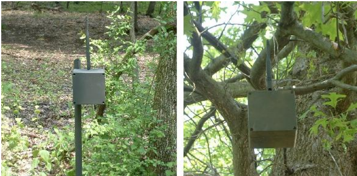
Figure 29. (Left) Camouflaged node enclosure on PVC pipe. (Right) Tree-hanging camouflaged node enclosure.
