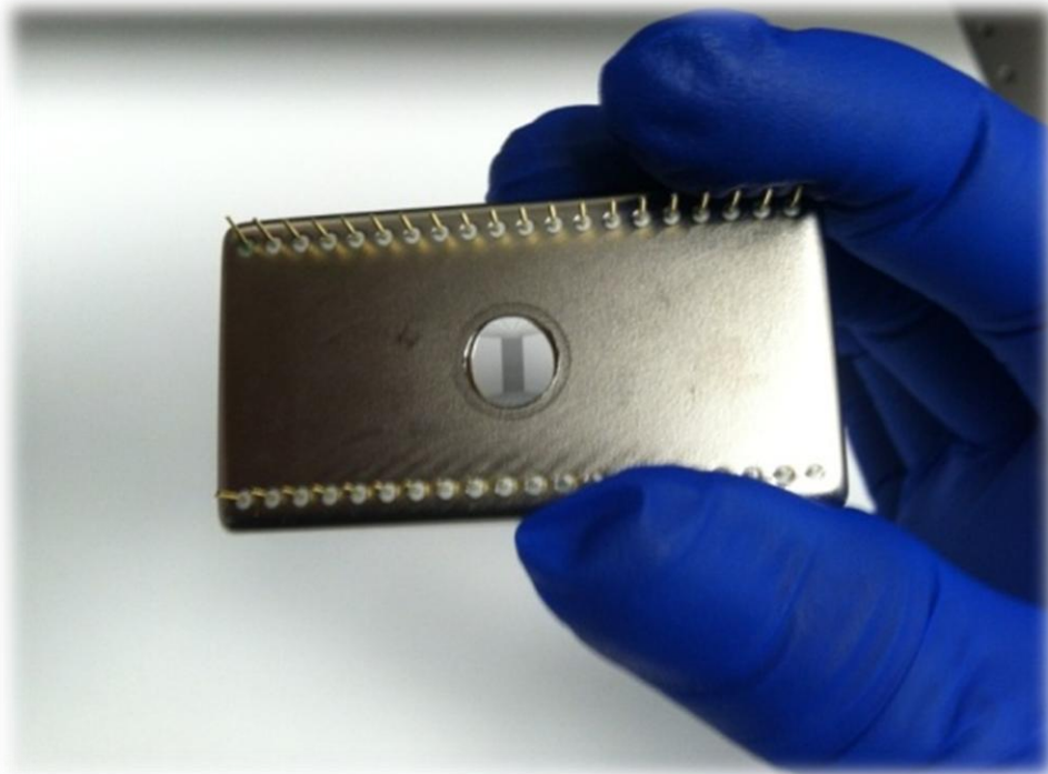
Figure 5.18 Hole drilled in back of package so that separation electrode array could be illuminated from its underside
