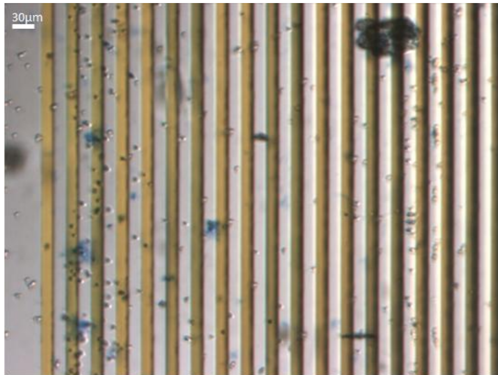
Figure 8.10 Top of figure shows initial distribution of cells in mixture containing live and dead yeast cells. Bottom of figure shows particles after 40 seconds of multiplexing between 100 kHz and 25 MHz. In this trial, the duration of each muxing cycle was shortened to 50us, short enough to average out the effects of the pDEP phase of the cycle
