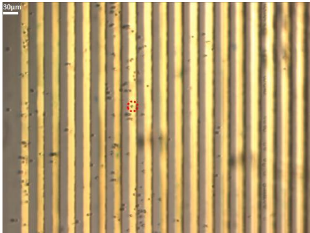
Figure 8.5 Top of figure shows initial position of a sample containing only live yeast cells. Bottom of figure shows position of cells after a 2Vpp, 100 kHz TWDEP field with a negative phase gradient is applied for 18s, resulting in an average lateral velocity of -6.7 \mu\text{m/s} .
