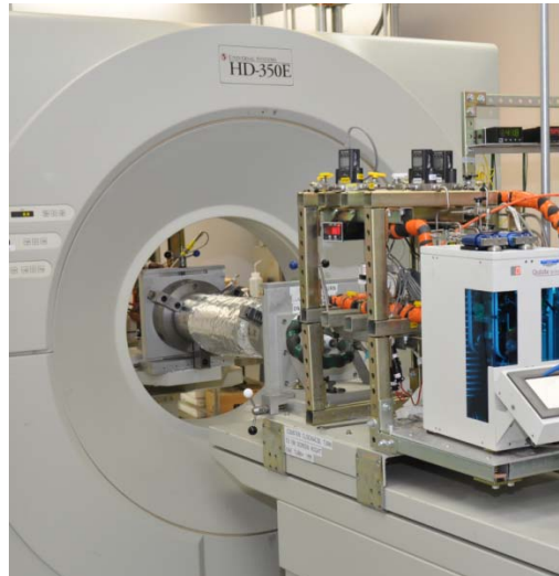
Figure 64. Medical CT scanner at NETL with core holder and flow pumps
