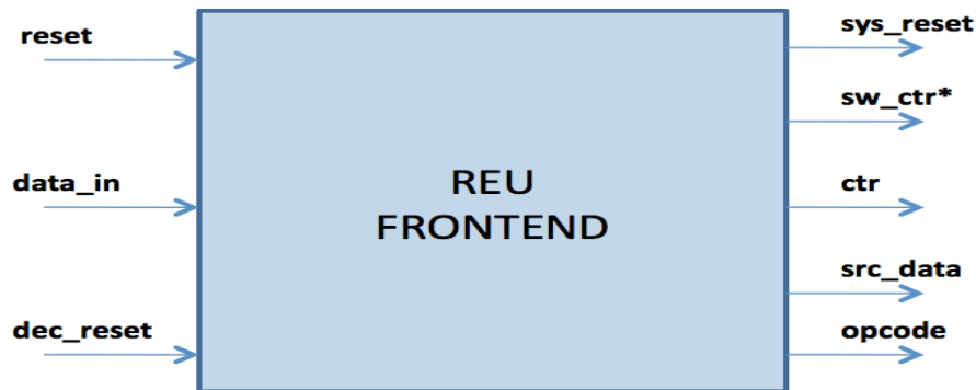
Figure 3.9: REU Frontend Pin Diagram
