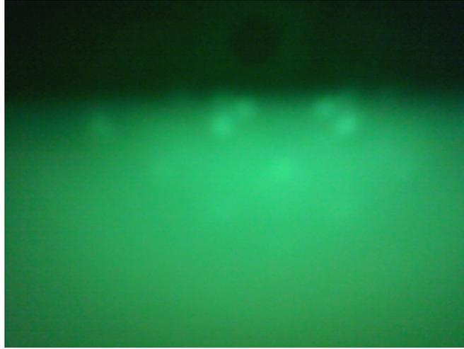
Figure 5.6 RHEED results for 10nm Si<sub>0.7</sub>Ge<sub>0.3</sub> growth on 6.5 nm Si buffer layer at 500 °C and 0.5
