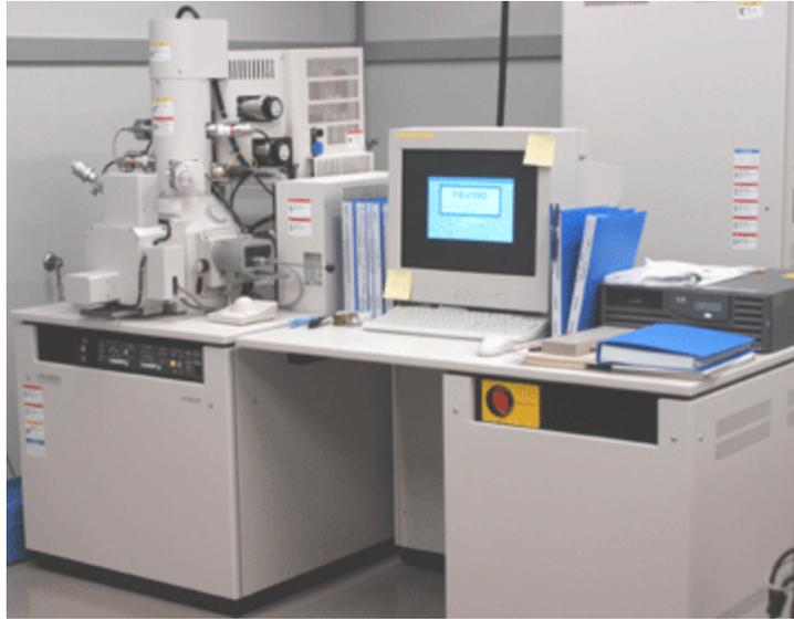
**Figure 2.2 Focused Ion Beam System.** <sup>68</sup>
