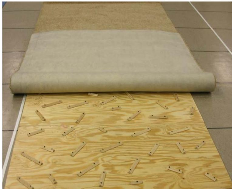
**Figure 10.** Walkway with an uneven surface.
