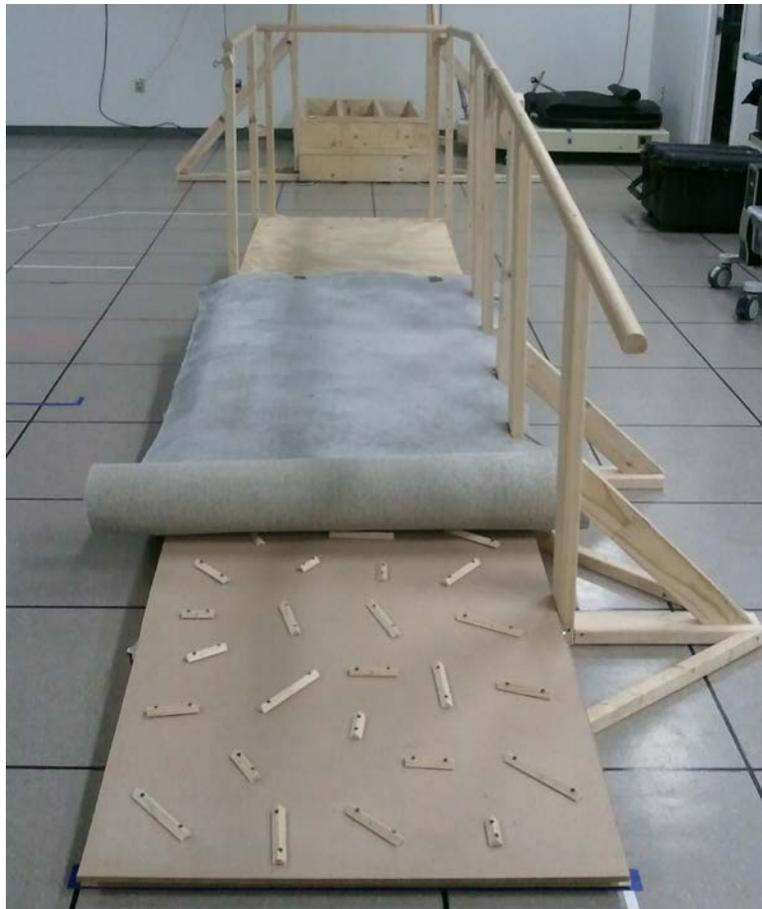
**Figure 9.** Ramp with a 5-degree incline and an uneven surface.
