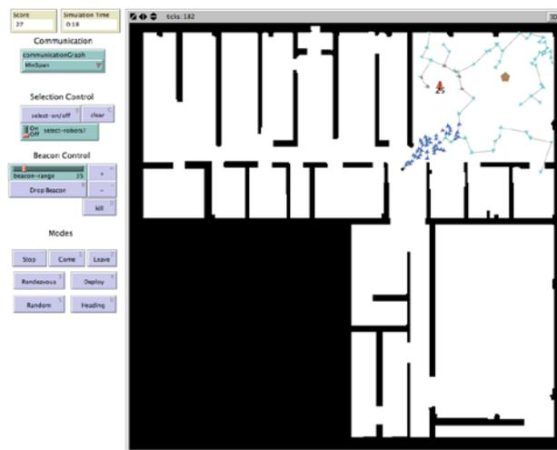
Figure 4. NetLogo interface for swarm experiments locations. For *beacon* control the operator could place, move, set the mode of, change the range of, and remove beacons. The heading mode requires an additional mouse click to determine the heading. For *selection* control the operator could select a rectangular set of robots, clear the current selection, and set the mode of all robots in the current selection. The come, leave and heading modes require an
