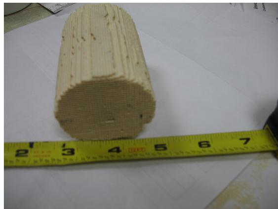
Figure 38: Regenerator used in the construction of the TAE.
