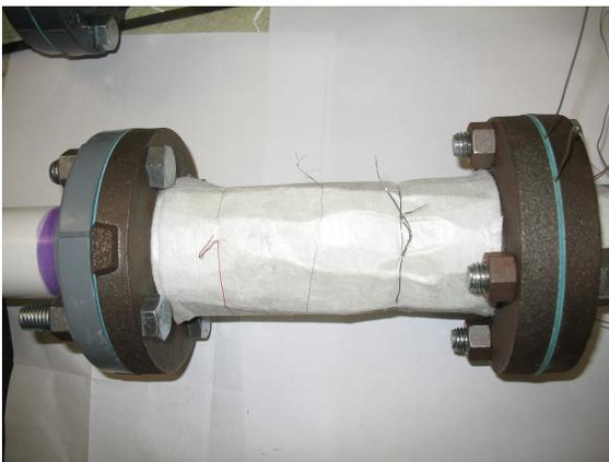
Figure 37: Housing design used to insure air tightness.
