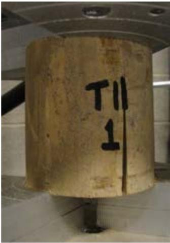
(b) Failure between shear planes
