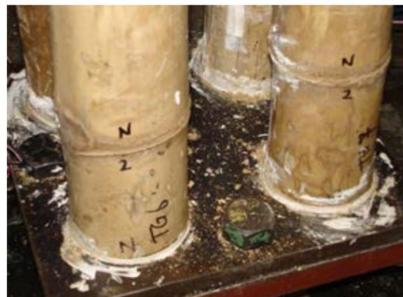
b) view of four-culm connection showing culms bearing on steel end plate
