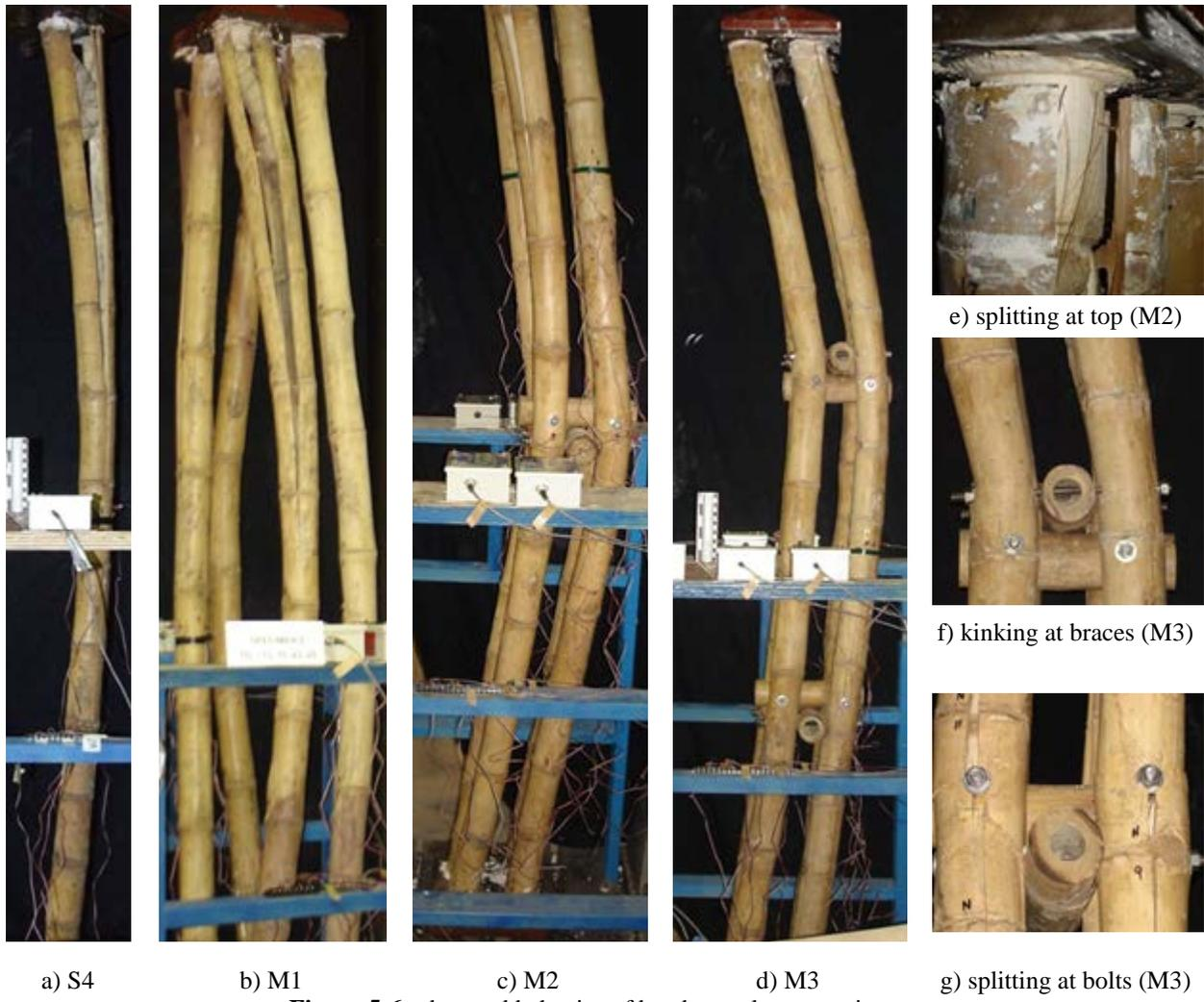
**Figure 5-6:** observed behavior of bamboo column specimens
