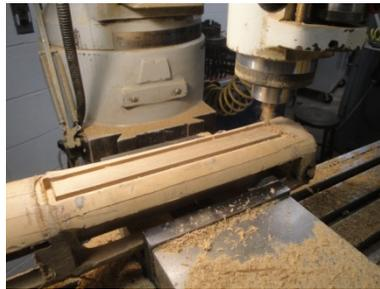
b) specimen fabrication in horizontal milling machine
