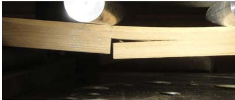
d) typical failure (Specimen T4 shown)
