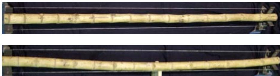
b) culms that are (top) relatively straight and (bottom) significantly curved in jig.
