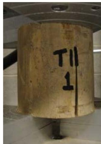
(b) Failure between shear planes
