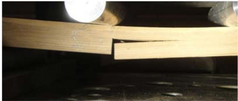
d) typical failure (Specimen T4 shown)
