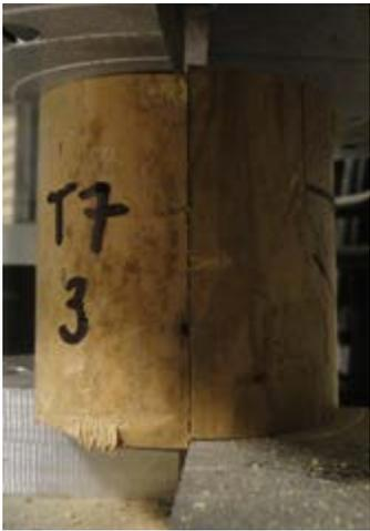
(a) Failure at shear plane
