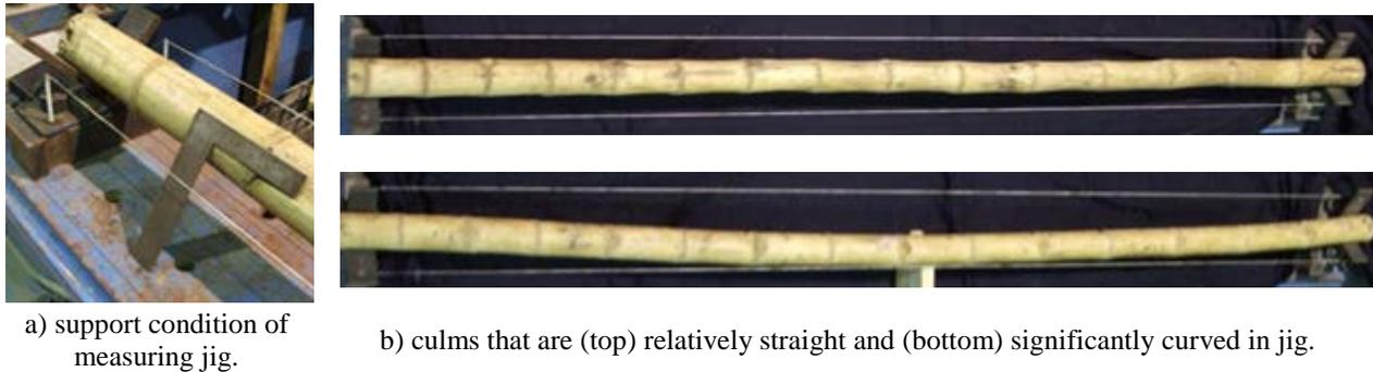
**Figure 5-1:** Jig for measuring bamboo columns
