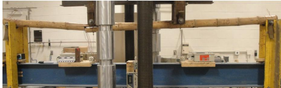
b) Notched specimen (T8) under load
