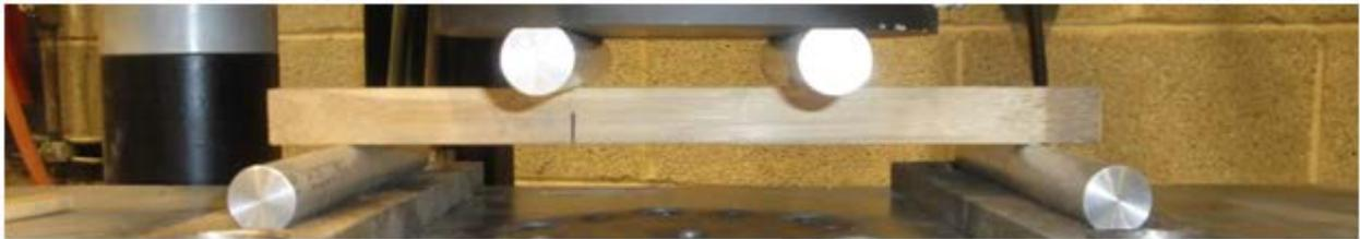
b) test set-up (Specimen T4 shown)
