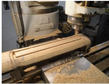
b) specimen fabrication in horizontal milling machine
