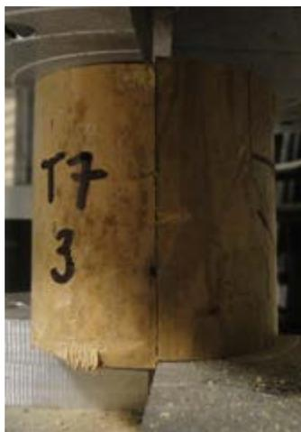
(a) Failure at shear plane
