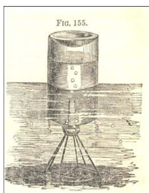
(left) Figure 26. Making light carbureted hydrogen ( Principles and Applications of Chemistry , 301)
