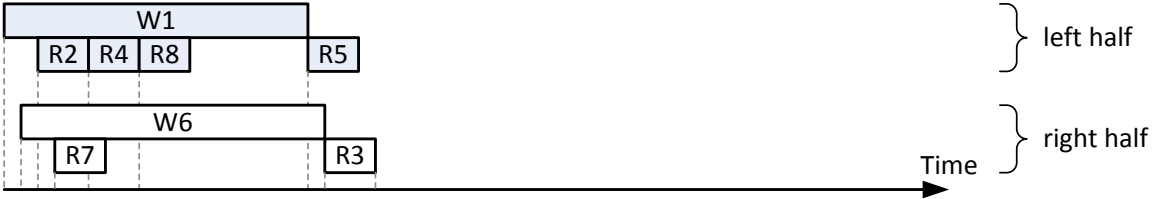
(c) Non-blocking Pseudo-Multi-Port Bank. Requests are issued out of order.
