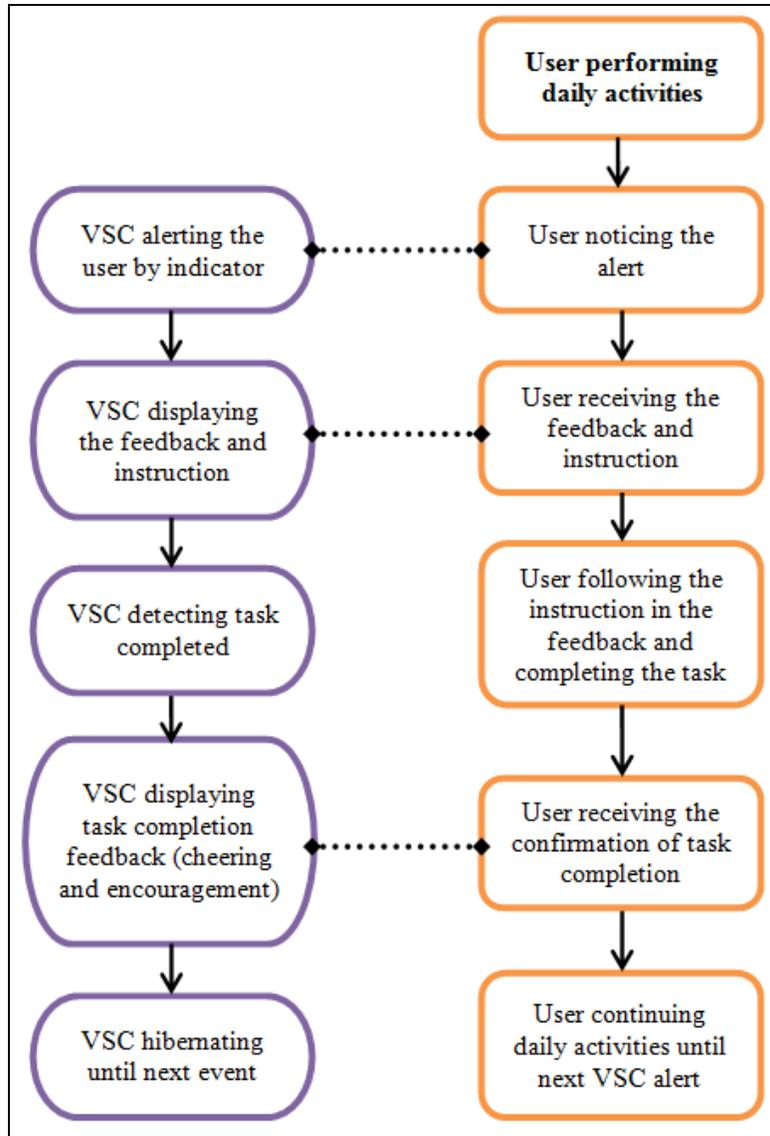
Figure 6. Interaction between the VSC and the user when the user was successfully following the coaching message.
