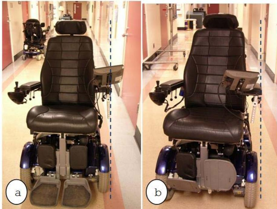
Figure 16. Improvement of the touch screen mount to decrease the width of the system and prevent equipment damage. The dash lines indicate the lateral edge of the wheelchair
