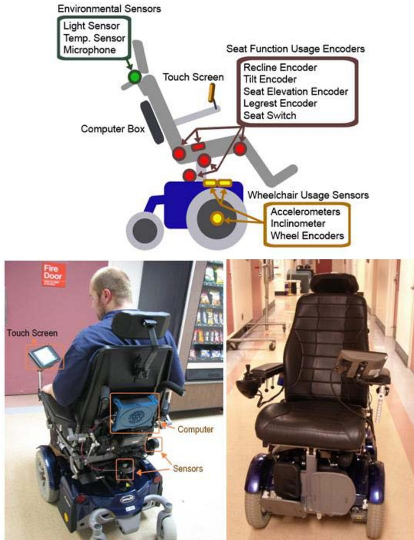
Figure 4. Instrumentation of Virtual Seating Coach System
