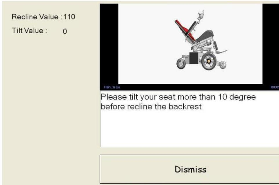
Figure 5. Prototype of VSC program
