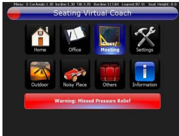
Figure 17. The red button indicates that there is an over-due pressure relief
