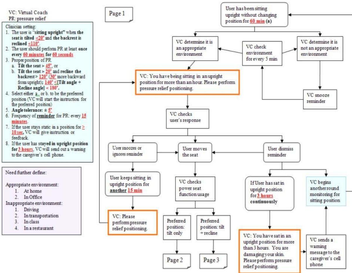
Figure 13. Example of VSC-User interaction flow chart to remind repositioning
