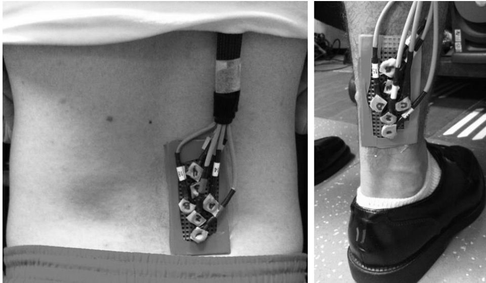
Figure 8: Erector spinae (left) and soleus (right) muscle NIRS probes placement.
