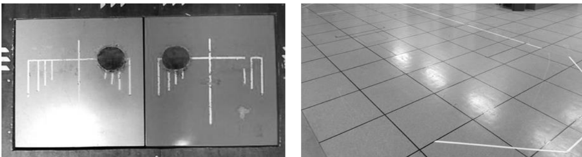
Figure 4: Hard flooring surface. (Left) Aluminum balance plate tile served as the hard flooring surface during standing sessions. (Right) Vinyl tile served as the hard flooring surface during walking sessions.
