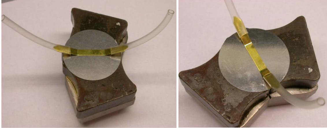
**Figure 7.5: Flow chamber mold prior to encapsulation in PDMS. The brass shim strip will produce the blood flow path and is glued to the stainless steel round shim disc on the bottom. The mold is pictured on top of the rare-earth magnet, used to stabilize the mold in the polystyrene dish as the PDMS is poured.**
