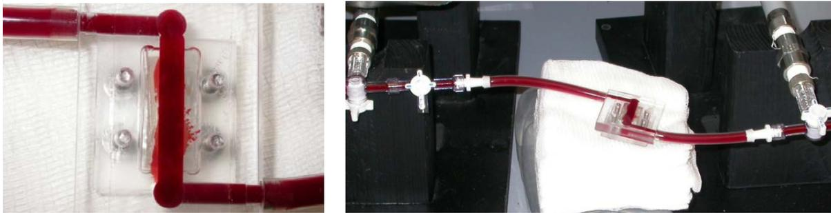
**Figure 7.12: Blood perfusion studies with the acrylic chamber. Left: blood leaking into imperfections in the glue between the acrylic chamber and the glass cover slip. Right: a sample material being exposed to flowing blood in the acrylic chamber.**
