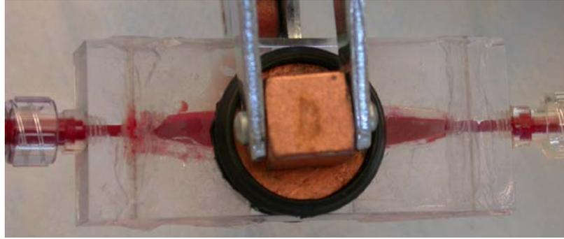
**Figure 7.3: The first generation polycarbonate parallel plate flow chamber following repair after breaking. Notice the rough edges of the flow path as well as the apparent leaks at the chamber junctions.**
