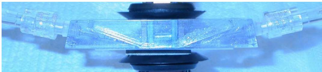
**Figure 7.2: The first generation polycarbonate parallel plate flow chamber clamped onto TiAl6V4 (bottom). A simple C-clamp provided the clamping pressure, and a silicon gasket was used to define the flow path width. Flow path height was not well controlled.**
