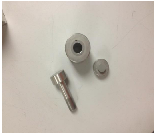
Figure 7 - Molding Dye Used for Pressing Silicon Carbide
