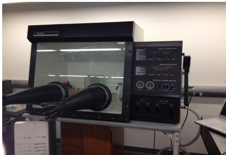
Figure 13 - Glovebox Used for Infiltration of Nickel Nanoparticles
