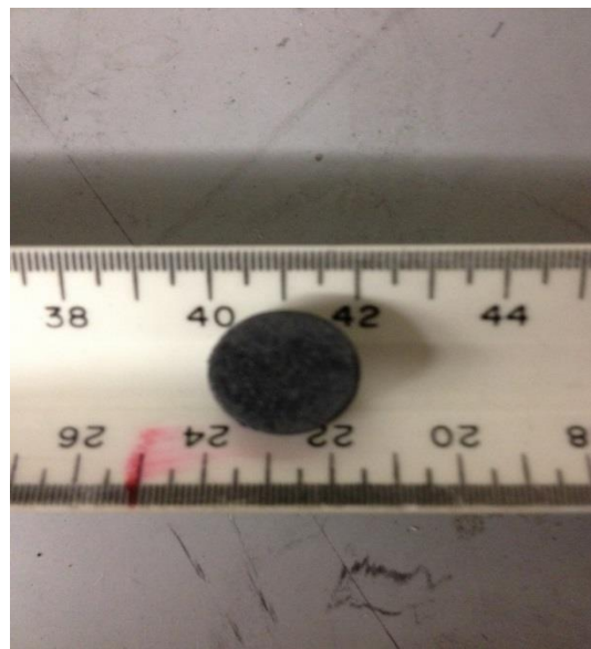
Figure 12 - 4 Time Infiltrated and Sintered Silicon Carbide Pellet
