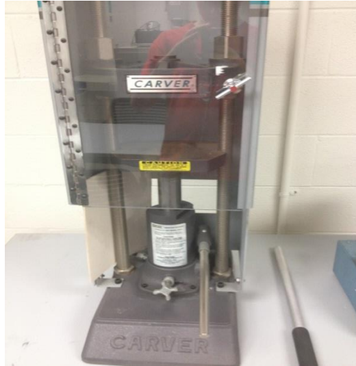
Figure 8 – Mechanical Pressing Machine for Compacting Silicon Carbide into Pellet Form
