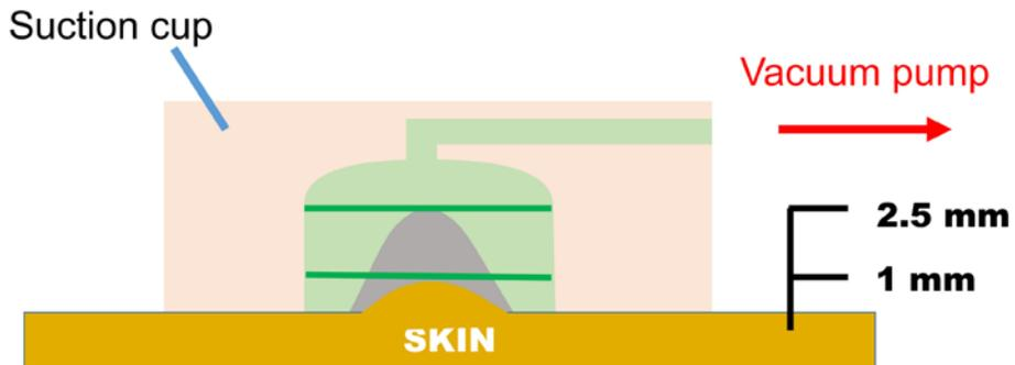
**Figure 3.1 A schematic demonstration of the DermaLab suction cup device**
