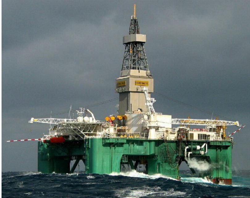
**Figure 1.2: Semi-Submersible Drilling Rig [7]**
