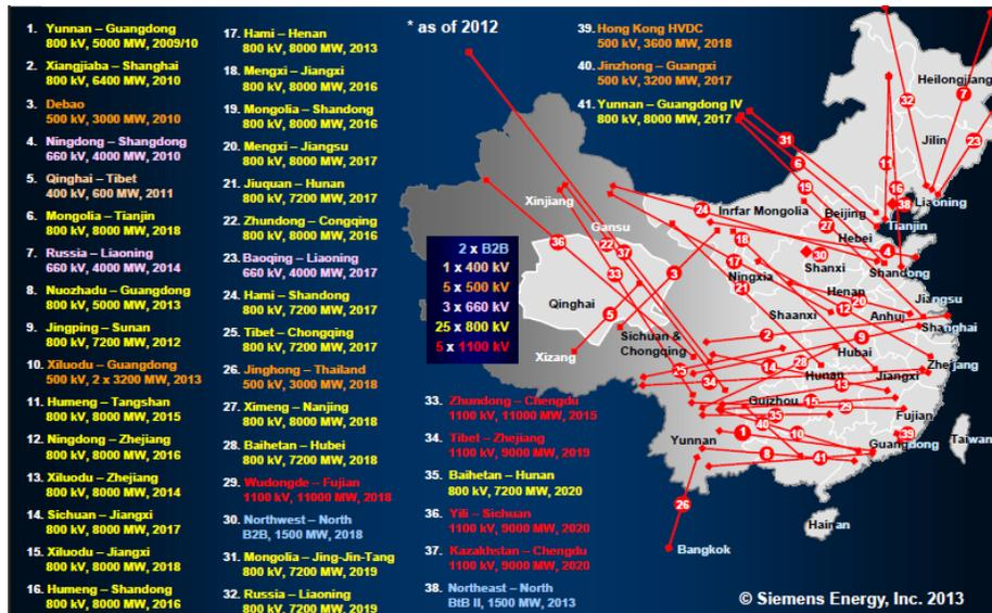
Figure 3.2: Planned HVDC Installations in China through 2020 [67]
