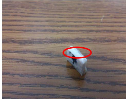
Figure 23: A brick shape sample cut off from the second part of the bone sample. Red painted region indicating the plane of interest (y direction).
