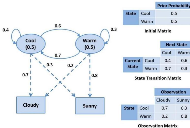
**Figure 5:** A weather system HMM with parameters
