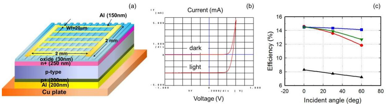
**Figure 3.20** (a) A Si n<sup>+</sup>pp<sup>+</sup>-junction (diffused) solar cell (b) I-V characteristic at 633 nm wavelength (7 mW, TE normal incidence): I<sub>sc</sub> = 2.94mA; V<sub>oc</sub> = 0.53V; FF = 0.71; efficiency = 15.7 %. (c) Efficiency vs incident angle: reference cell (planar with oxide) (black); 1D mesa & oxide (TE/TM avg) (red); 1D mesa & oxide (TE'/TM' avg) (blue); 2D mesa & oxide (green).
