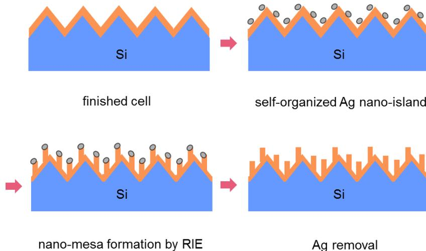
**Figure 4.4** A non-lithographic manufacturing process for self-aligned vertical dipole structures.
