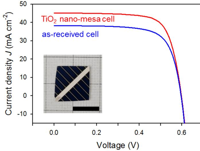
**Figure 5.5** I-V characteristics of a reference cell and a TiO<sub>2</sub> nano-mesa cell.
