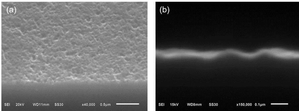
**Figure. 5.2** SEM images of nano-mesas using  $\text{TiO}_2$  masks.
