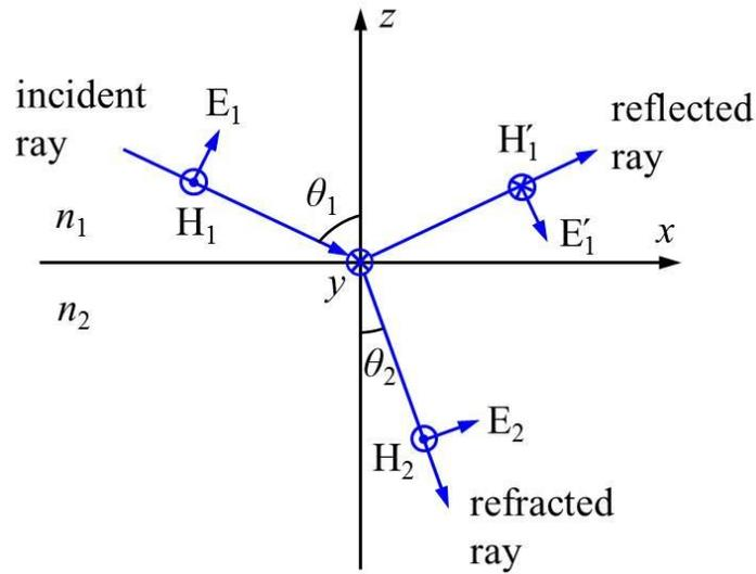
**Figure 3.6** Reflection and refraction waves at an interface of two dielectric media.
