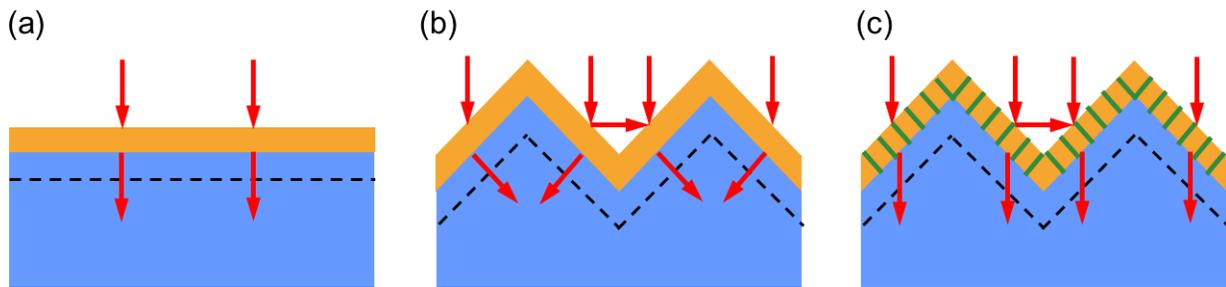
**Figure 4.1** Schematic of light propagation on (a) planar surface, (b) pyramid-textured surface, (c) pyramid-textured surface with vertical dipoles.
