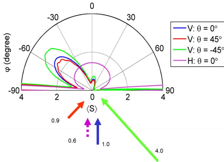
**Figure 2.5** Radiation patterns of a vertical nanoslit calculated at three different incident angles. The transmission throughput ratio is marked by the arrow length.
