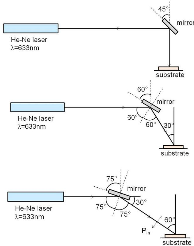
**Figure 3.18** Optical set-up for measuring angular dependence of efficiencies.
