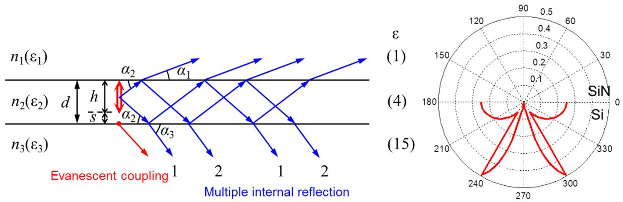
**Figure 2.7** Radiation patterns of a vertical dipole embedded in the passivation layer of a Si cell.
