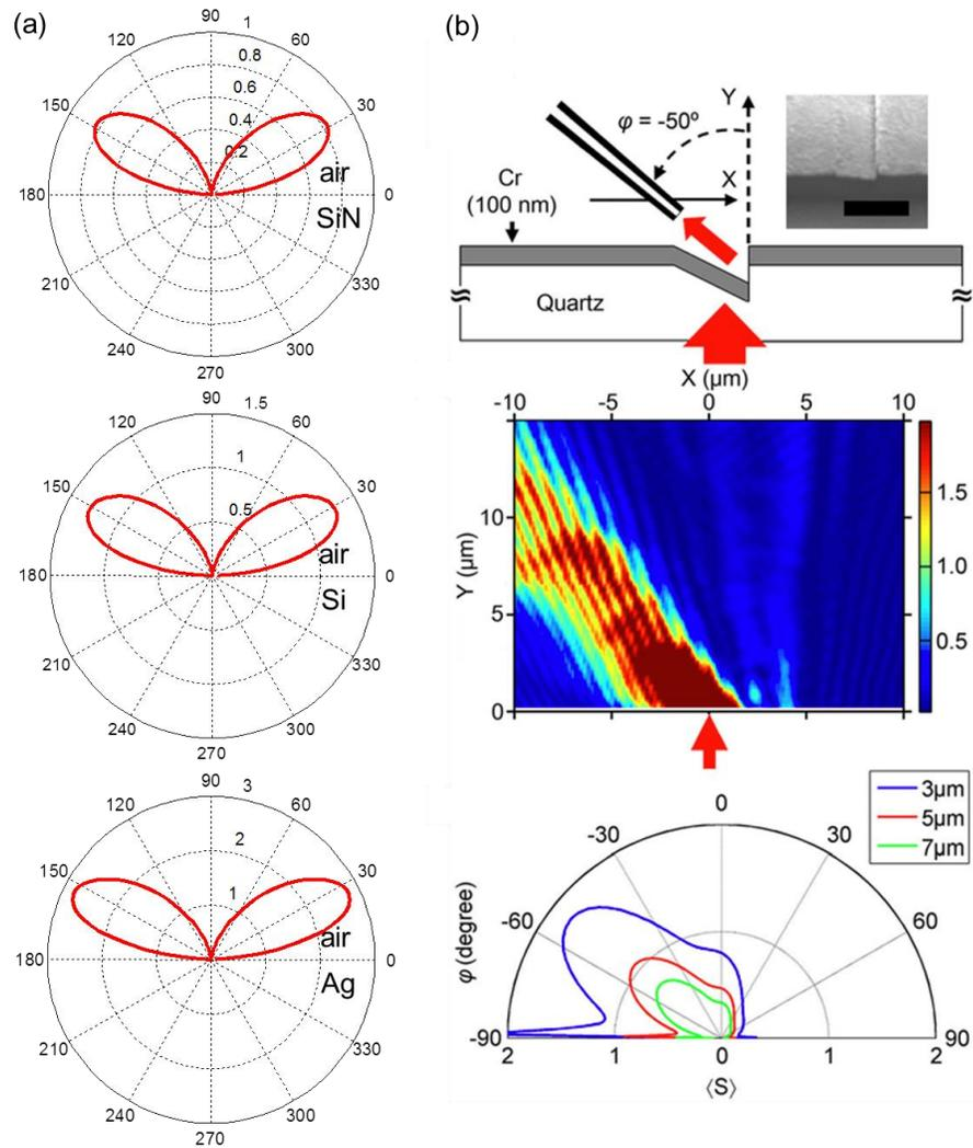
**Figure 2.3** (a) Radiation patterns in the air side calculated for three different media, SiN, Si and Ag at 633nm wavelength. (b) Scanning probe measurement of radiation pattern of a vertical nanoslit formed in Cr film (top), radiation pattern measured at 633 nm wavelength (middle), FDTD simulation of radiation patterns at three different radial distances from the aperture center.
