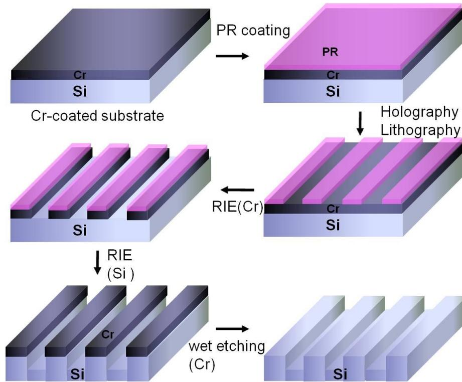
**Figure 3.3** Schematic of fabricating gratings using holographic lithography.
