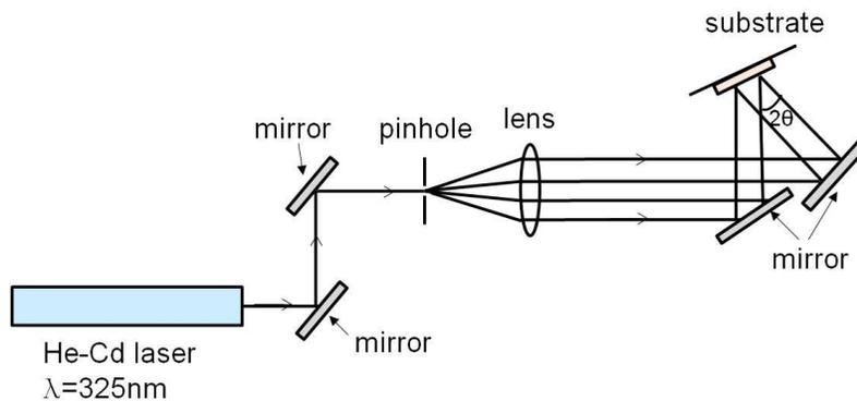
**Figure 3.1** Schematic of holographic lithography setup.
