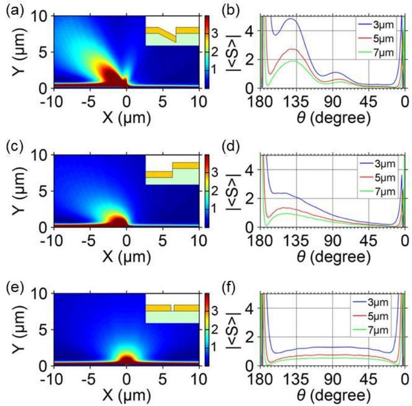
**Figure 2.4** FDTD calculation of optical transmission through vertical nanoslit structures. Radiation patterns of Ag nanoslits (gap size: 60 nm). (a)-(d) Vertical nanoslit structures (inset: cross-section). The main lobes are tilt-oriented to 50-60° direction. (e),(f) Conventional horizontal nanoslit.
