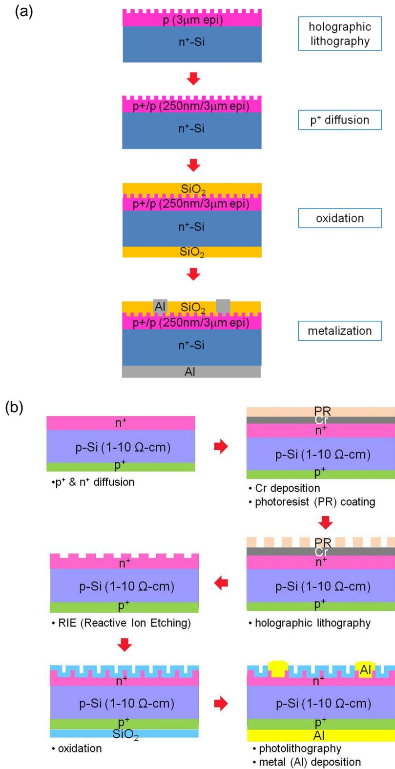
**Figure 3.5** Schematic of fabrication process for (a) a Si pn-junction (p-epitaxial) solar cell (b) a Si n<sup>+</sup>pp<sup>+</sup>-junction (diffusion) solar cell.
