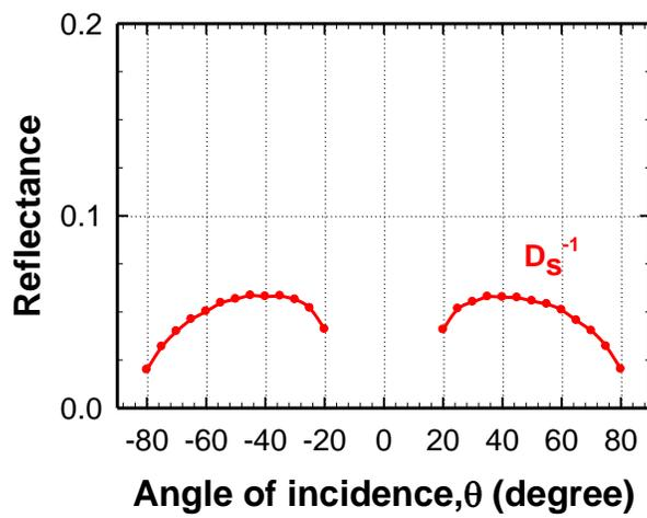
**Figure 3.14** Angular dependence of reflectance when the grating period  $d = 500$  nm and  $\lambda = 633$
