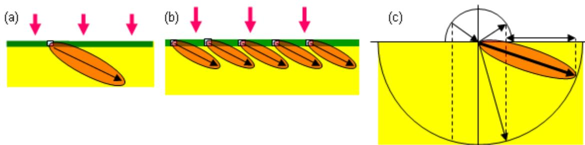
**Figure 2.2** (a) Highly-directed radiation pattern of a vertical dipole nanoaperture. (b) Radiation from an array of nanoaperture. (c) Phase matching condition for glancing angle transmission through a nanoaperture array.
