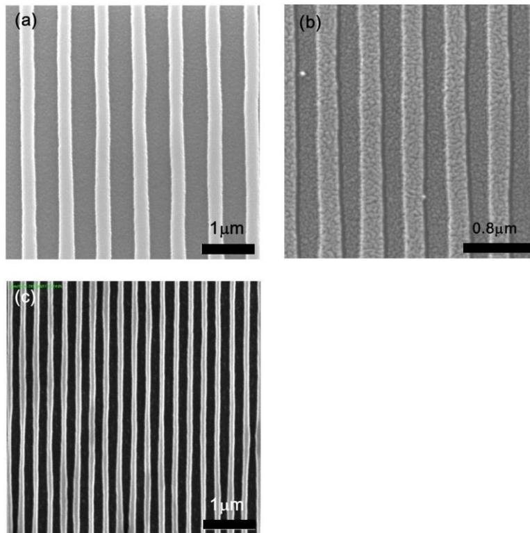
**Figure 3.4** SEM images of gratings with (a) 720, (b) 500 and (c) 270 nm period.
