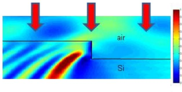
**Figure 3.9** FDTD simulation of light transmission through a single vertical nano-step surface of Si: step height, 220 nm; normal incidence of 633 nm, TM polarized light. Glancing angle transmission mediated by vertical dipole excitation is clearly visible.
