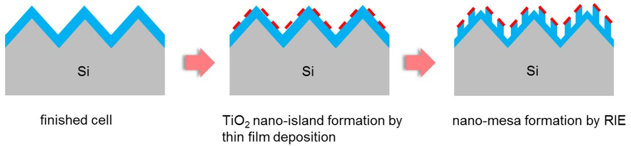
**Figure 5.1** Fabrication process scheme of TiO<sub>2</sub> nano-mesa structure.
