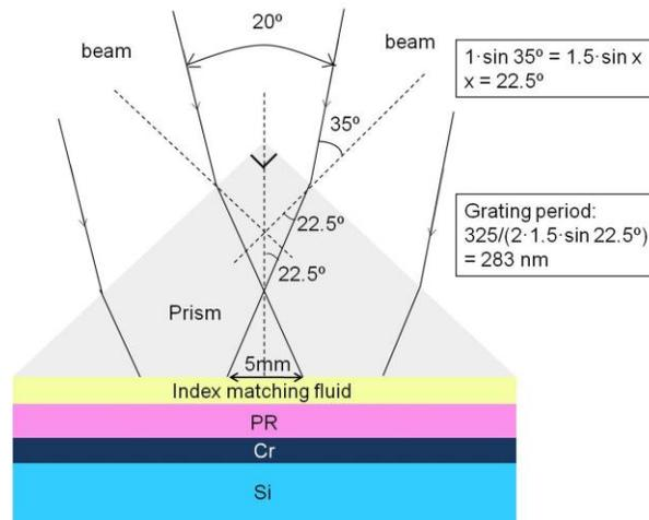
**Figure 3.2** Schematic of exposure through a prism.
