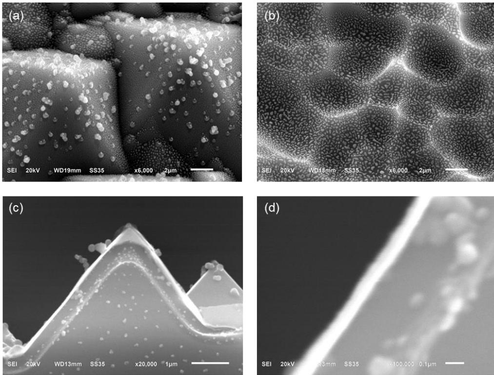
**Figure 4.5** SEM images of commercial cells with Ag nanoislands. (a) ML Solar c-Si (b) Everbright mc-Si (top view) (c), (d) c-Si pyramidal textured cell (cross-sectional view).
