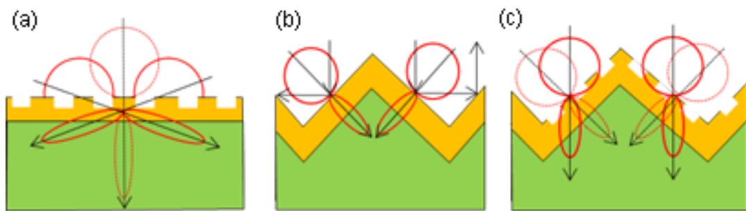
**Figure 4.2** Coupling of light into Si: (a) planar surface with nano-vertical steps; (b) pyramid-etched surface; (c) pyramid surface textured with nano-vertical steps. Note nano-vertical dipoles enable glancing coupling of light.
