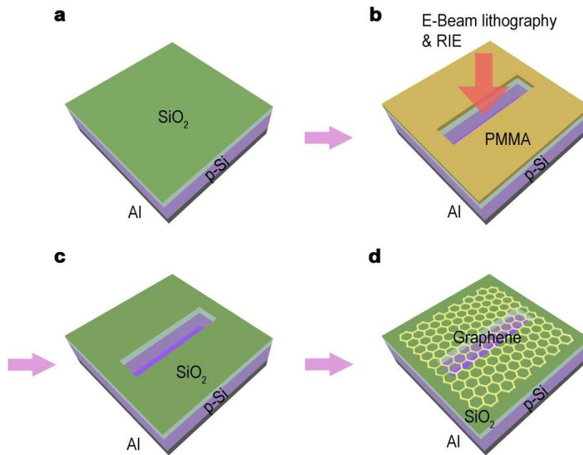
**Figure 6.1** Schematic of fabrication process of the graphene/SiO<sub>2</sub>/Si structure.
