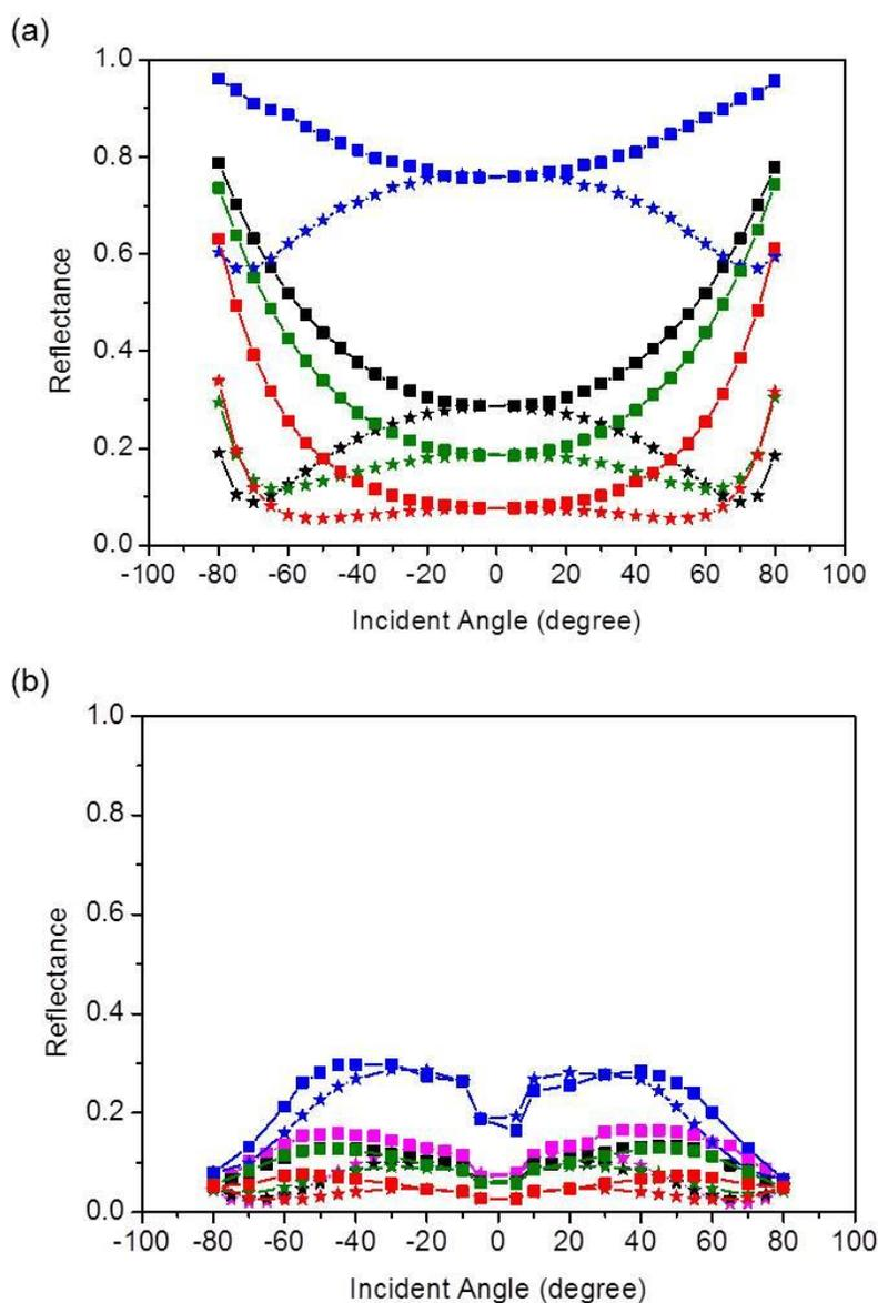
**Figure 4.7** Reflectance measurement of Ag nano-steps formed on planar and pyramidal Si at 633 nm wavelength (a) planar Si with oxide (TE/TM) (black); 24 nm Ag deposition (TE/TM) (blue); Ag annealing (TE/TM) (green); removal of Ag (TE/TM) (red). (b) pyramidal Si (TE/TM) (pink); pyramidal Si with oxide (TE/TM) (black); 24 nm Ag deposition (TE/TM) (blue); Ag annealing (TE/TM) (green); removal of Ag (TE/TM) (red). The reflectance of panel (b) is with arbitrary unit and uncalibrated.
