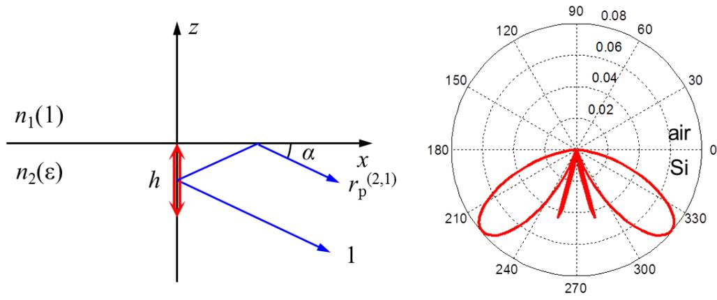
**Figure 2.6** Radiation patterns of a vertical dipole placed underneath a dielectric surface.
