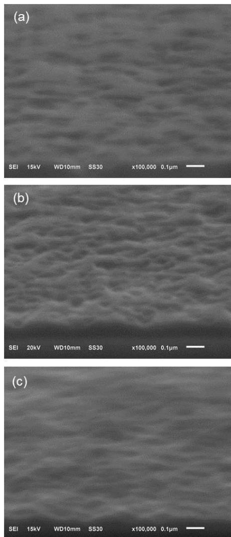
**Fig. 5.3** SEM images of  $\text{TiO}_2$  nanoislands depending on the etching time. (a) less-etching (b) optimum-etching (c) over-etching.
