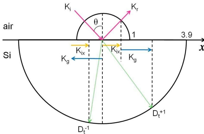
**Figure 3.12** Phase matching diagram between air and silicon.
