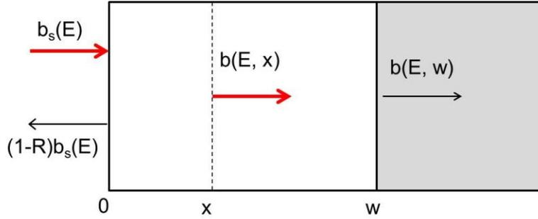
**Figure 1.3** Attenuation, transmission and reflection of incident light in a semiconductor layer of active width  $w$ .
