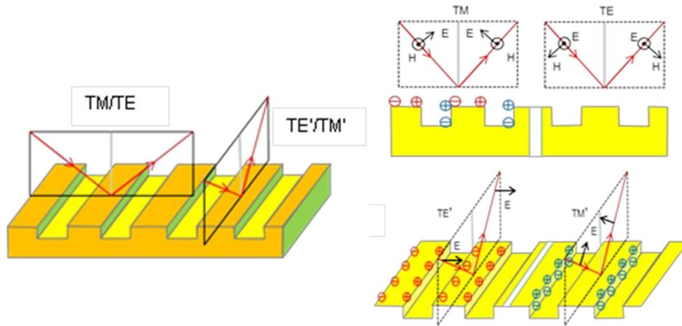
**Figure 3.8** Four possible configurations of beam polarization incident to a 1D grating. Reflectance spectra measured at 633 nm wavelength on thin-film Si vertical-mesa array (bottom left) and planar Si surface (bottom middle). Vertical dipoles (blue) and horizontal dipoles (red) are marked on mesa facets (right).
