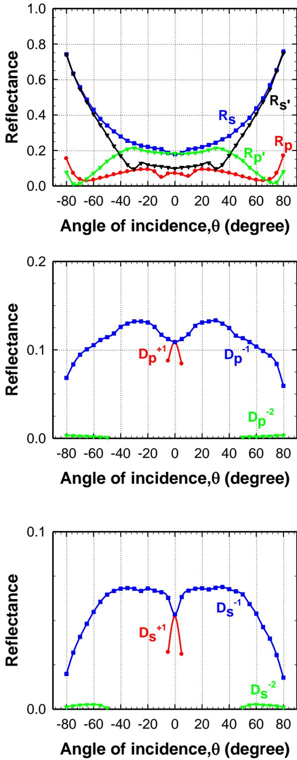
**Figure 3.13** Angular dependence of reflectance when the grating period  $d = 720$  nm and  $\lambda = 633$
