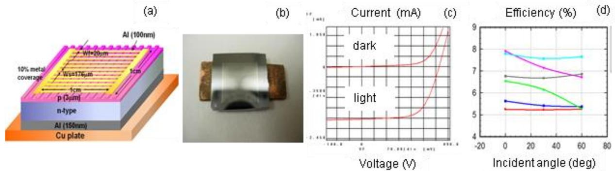
**Figure 3.19** (a),(b) A prototype Si pn-junction solar cell fabricated in this study. (c) I-V characteristic at 633 nm wavelength (6.85 mW, TM normal incidence):  $I_{sc} = 1.85\text{mA}$ ;  $V_{oc} = 0.42\text{V}$ ;  $FF = 0.7$ ; efficiency = 7.95 %. (d) Efficiency vs incident angle: reference cell (planar without oxide) (red); planar with oxide (blue); mesa without oxide (TE/TM) (green); mesa without oxide (TE'/TM') (grey); mesa & oxide (TE/TM) (purple); mesa & oxide (TE'/TM') (light blue).
