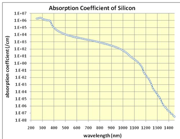
**Figure 1.1** Reflectivity and absorption coefficient of silicon. [2]
