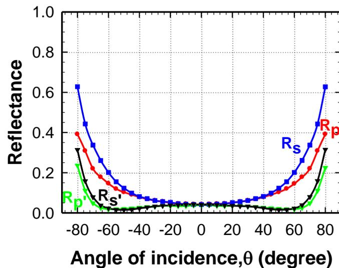
**Figure 3.17** Angular dependence of reflectance when the grating period  $d = 270$  nm and  $\lambda = 633$  nm with an oxide layer.
