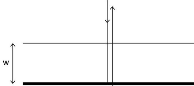
**Figure 1.5** Double path-length in a rear mirror cell.
