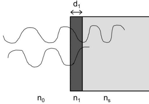
**Figure 1.4** Single layer AR coating.
