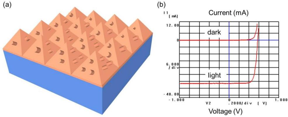
**Figure 4.8** Nanoscale vertical dipole on a finished cell. (a) Schematic of nano-texture on pyramid cell. (b) I-V curves showing dark and photocurrent.
