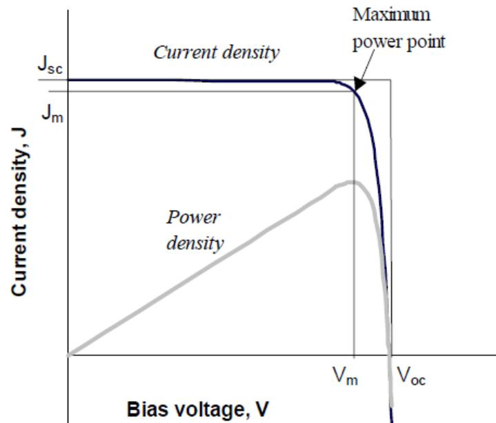
**Figure 1.8** Current versus voltage graph showing open-circuit voltage ( $V_{oc}$ ), short-circuit current ( $I_{sc}$ ) and fill factor (FF) [21].
