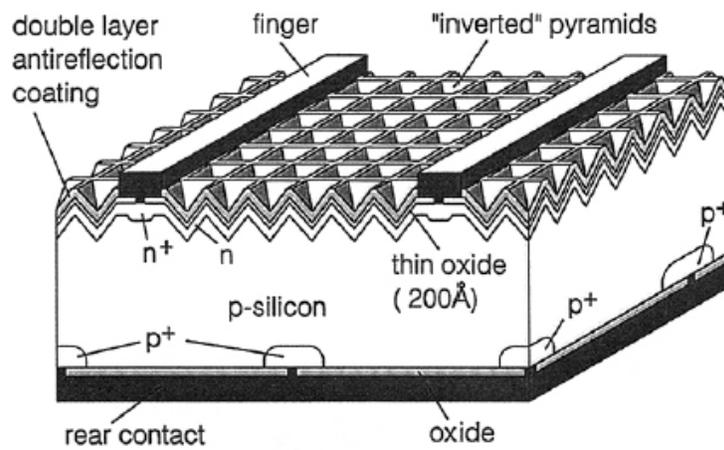
**Figure 1.2** The typical PERC (passivated emitter, rear locally-diffused) cell with the efficiency of 24%. [20]
