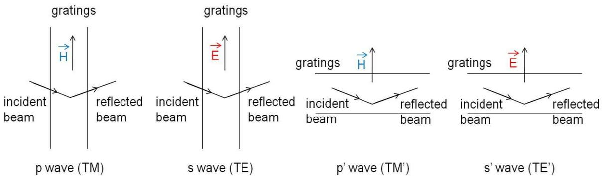
**Figure 3.7** Four configurations of our optical measurement.
