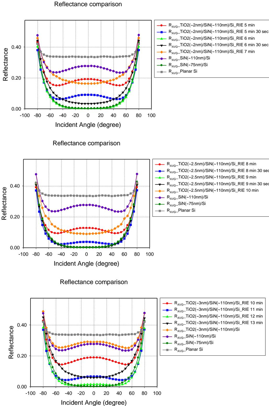
**Figure 5.4** Reflectance measurements of 2, 2.5 and 3 nm-thick TiO<sub>2</sub> nanofilms on SiN/Si substrate after RIE at 633 nm wavelength.
