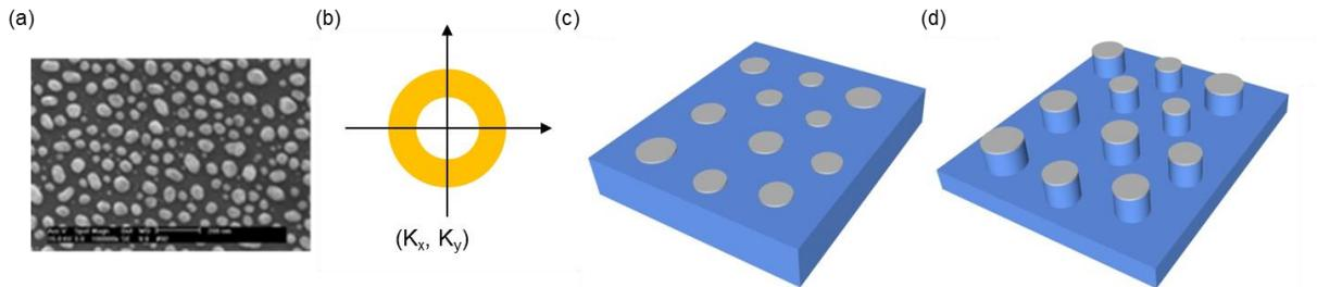
**Figure 4.3** (a) SEM image of Ag nano-disks formed on silica surface. (b) Grating vector distribution of the Ag nano-particle array. (c)&(d). A schematic of fabricating nano-vertical steps: Self-organized metal nano-disks are used as an etch mask in plasma or chemical etching of silica or Si.
