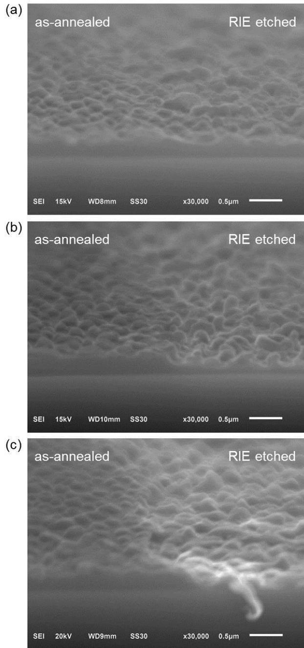
**Figure 4.9** SEM images of reactive etching profile of Ag nanoparticles on SiN. Left: as-annealed Ag, Right: RIE treated Ag (a) RIE 1 min (b) RIE 2 min (c) RIE 3 min.
