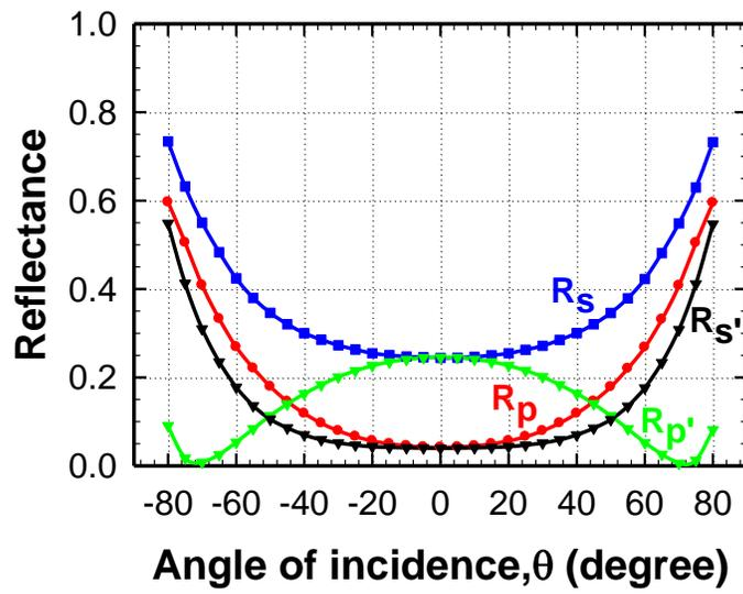
**Figure 3.16** Angular dependence of reflectance when the grating period  $d = 270$  nm and
