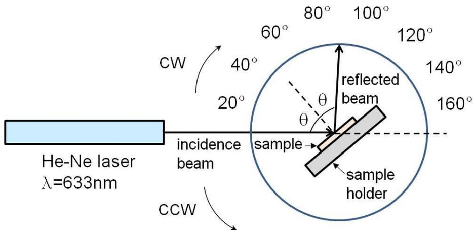
**Figure 3.10** Scheme of optical measurement to characterize the angular dependence of reflection.
