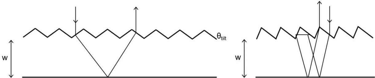
**Figure 1.7** (a) Reflection path in a symmetrically textured surface (b) Four passes of light in an asymmetrically textured surface.
