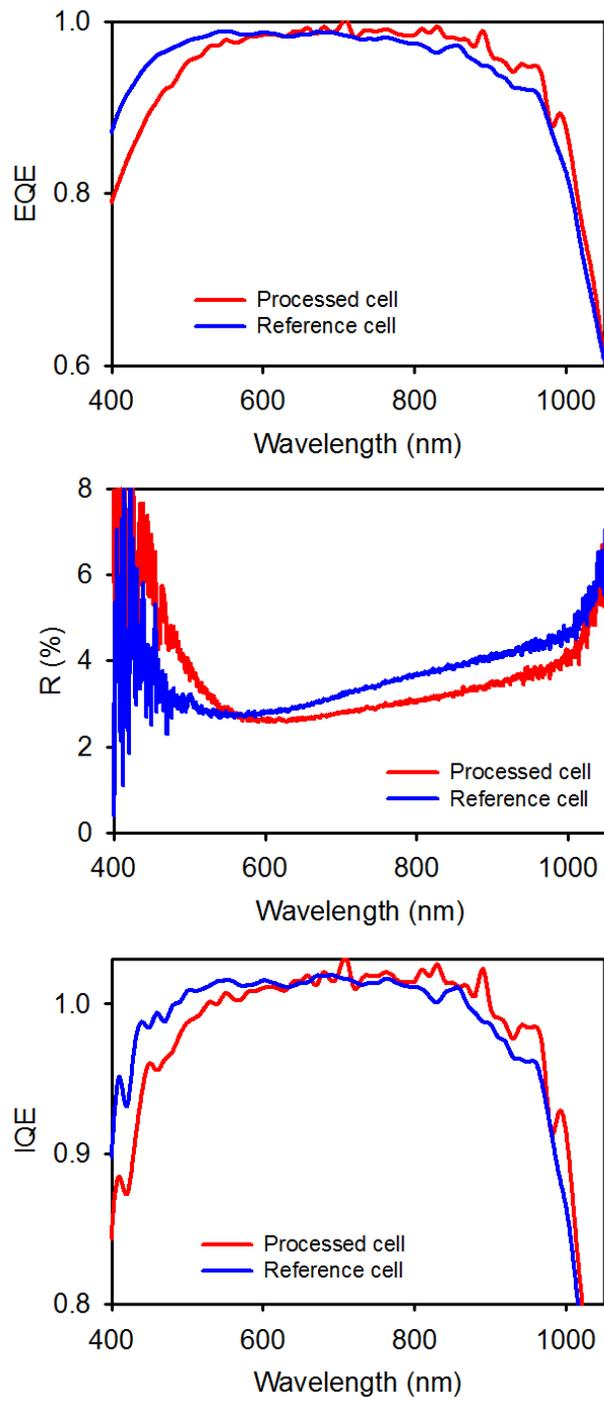
**Figure 5.6** Measured reflectance, EQE and IQE spectra of c-Si cells with and without vertical dipoles.
