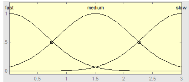
Figure 3. Membership Function for Input Variable "Press-Time"
