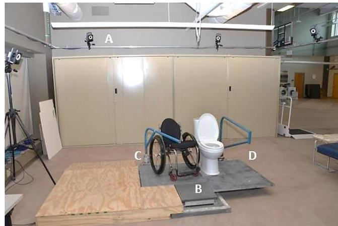
**Figure 4.** The transfer station includes a 10-camera Vicon Nexus motion analysis system (Vicon, Centennial, CO) (A), three force plates under the wheelchair, subjects' feet, and the toilet (Bertec Corporation, Columbus, OH) (B), and two load cells (Model MC5 from AMTI, Watertown, MA; Model Omega 160 from ATI, Apex, NC) attached to the two grab bars respectively (C and D).
