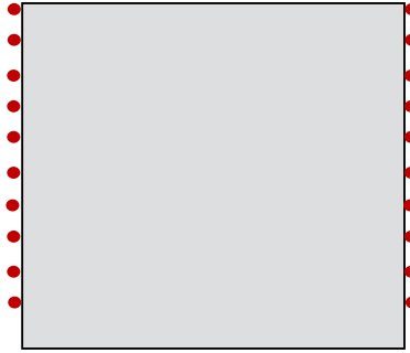
Figure 3.8: Schematic of the horizontal and vertical displacement sensor locations (red dots) for Example 2: Simulated Hard Matrix with Soft Inclusions.
