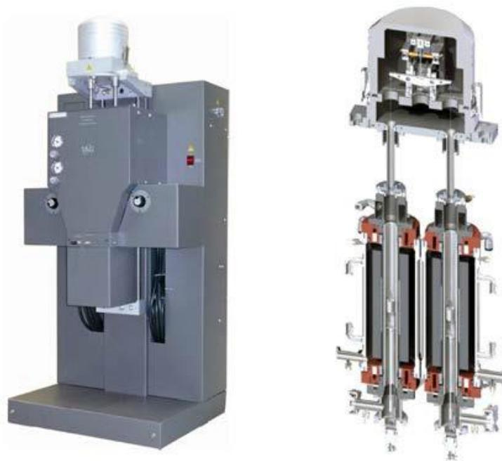
Figure 3.1 Setaram high performance symmetrical TAG system
