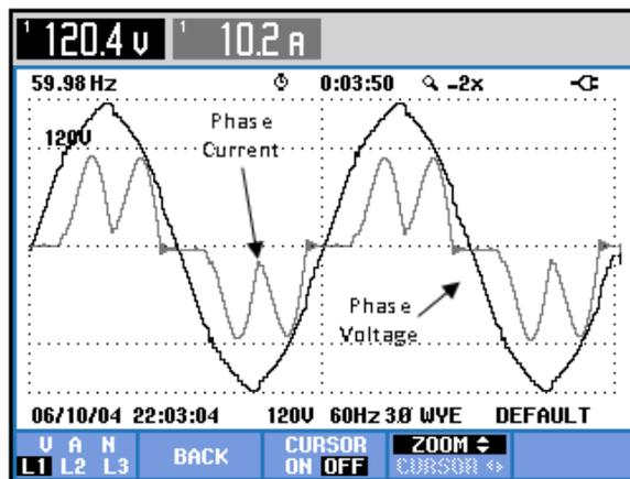
**Figure 67.** Current and voltage waveforms associated with phase A of the VFD
