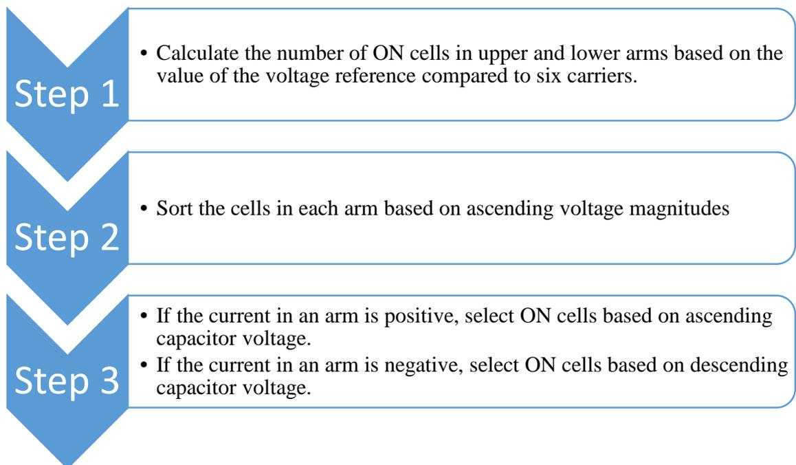
**Figure 52:** Overview of Capacitor Balancing Process
