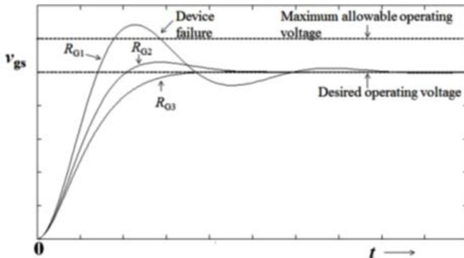
**Figure 3.** Turn-on characteristic.  $R_{G1} < R_{G2} < R_{G3}$
