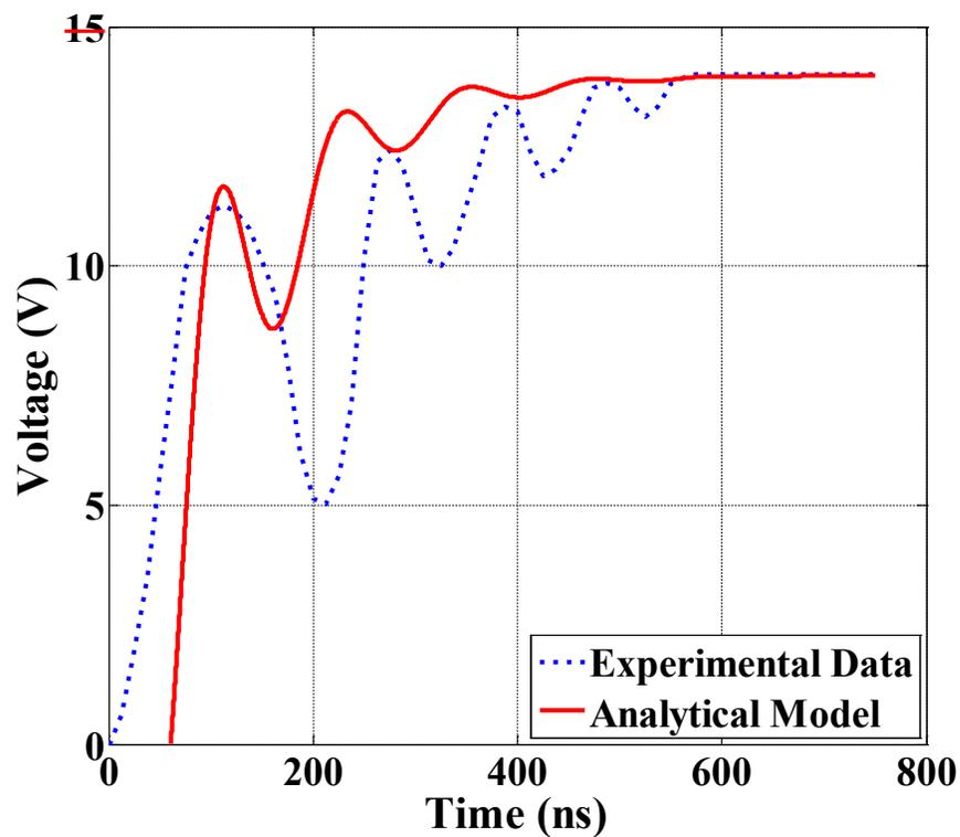
**Figure 18.** Analytical step response for  $v_{gs1}$  compared with experimental  $v_{gs1}$
