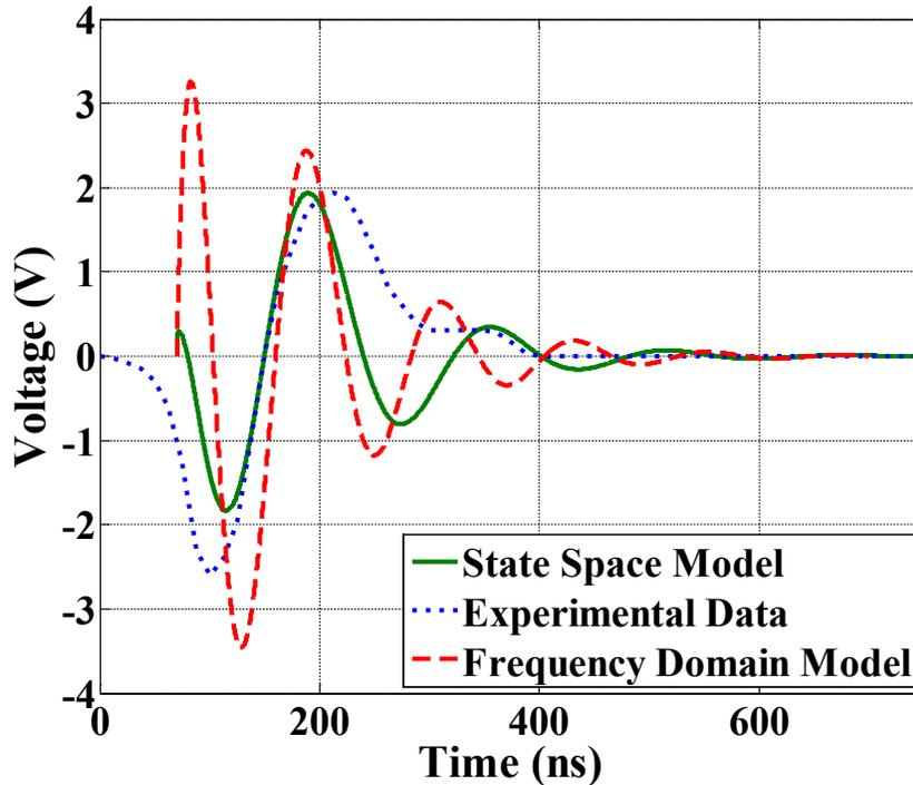
**Figure 24.** Turn-on response for  $v_{gs2}$
