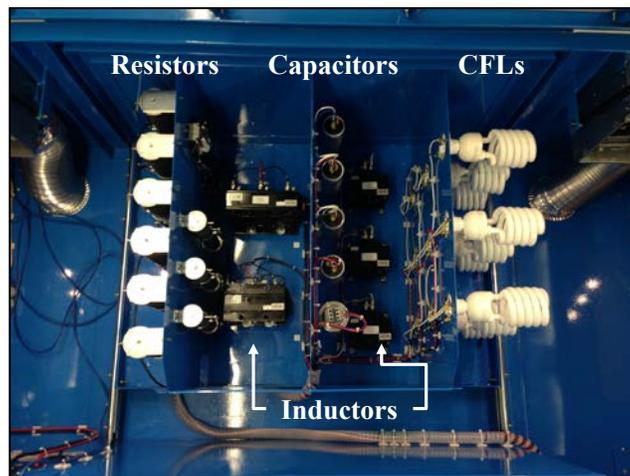
**Figure 63.** Internal top-down view of workbench
