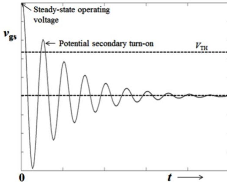
**Figure 5.** Turn-off characteristic of a device
