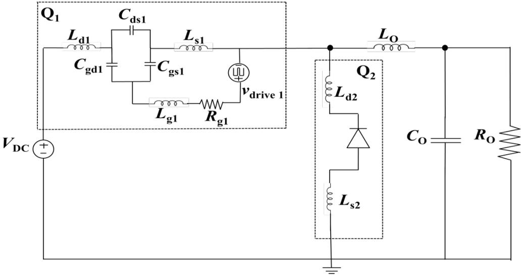
**Figure 14.** Synchronous buck converter during dead time interval
