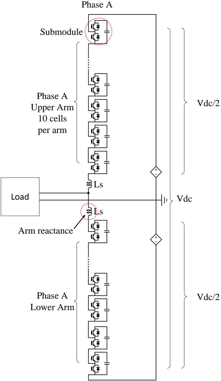
**Figure 50.** Single phase MMC inverter topology
