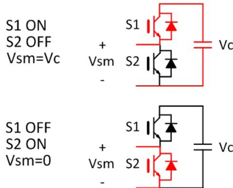
**Figure 49.** Submodule operation of MMC showing primary switching states
