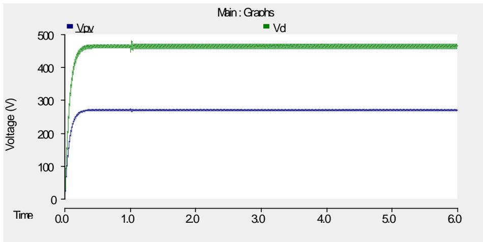
**Figure 38.** Test Condition I: input and output voltage waveforms
