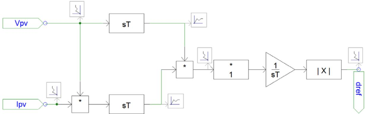
**Figure 35.** RCC implementation in PSCAD
