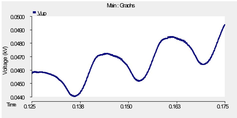
**Figure 56.** Voltage drift on upper arm capacitor without balancing control
