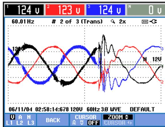
**Figure 66.** Trapped charge voltage transient on the capacitor bank
