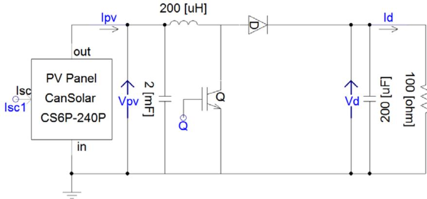
**Figure 34.** Simulated PV panel and boost converter system
