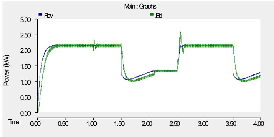
**Figure 47.** Test Condition III: input and output power waveforms
