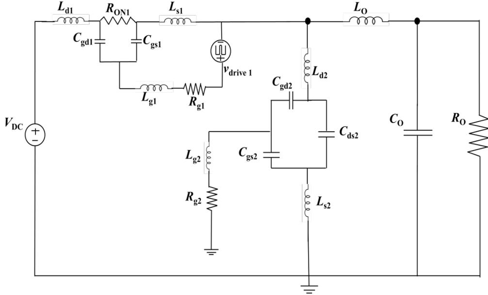
**Figure 15.** Equivalent circuit for the converter immediately after formation of  $Q_1$  channel
