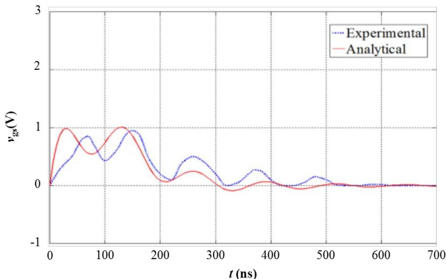
**Figure 11.** Analytical and experimental induced gate-source voltage with  $C_{GS} = 30$  nF
