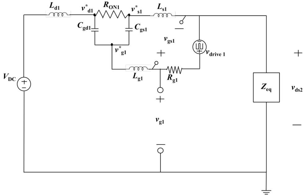
**Figure 16.** Simplified version of Figure 15 with node voltages indicated for  $Q_1$
