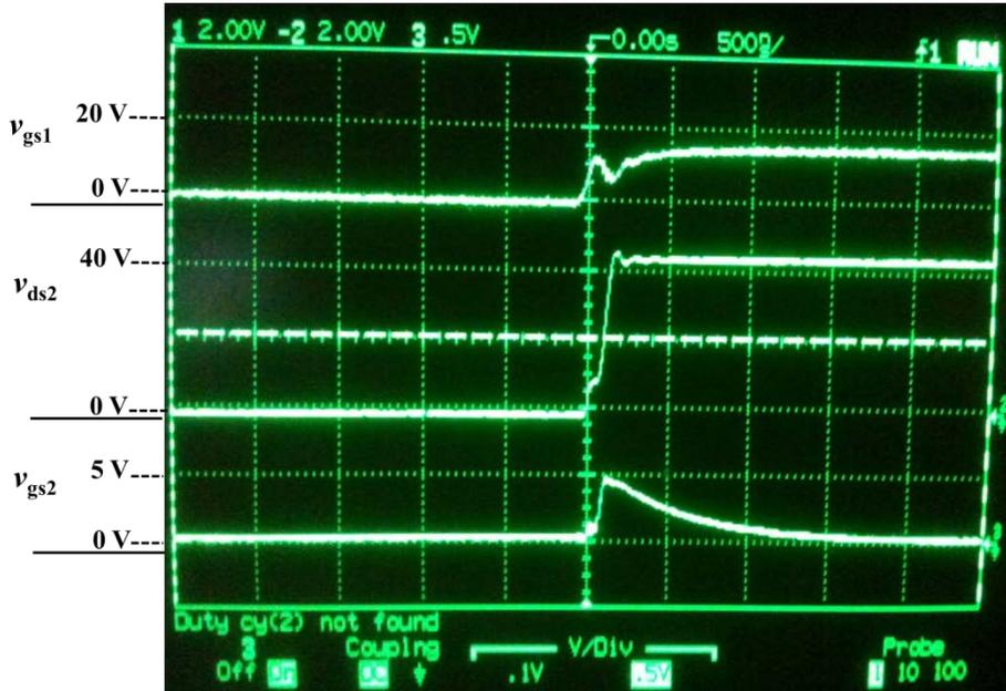
**Figure 25.** Experimental waveforms after  $R_{g2}$  is raised to  $45 \Omega$ . 10:1 testing probes were used for measurement, while the scope measurement is set to 1:1.
