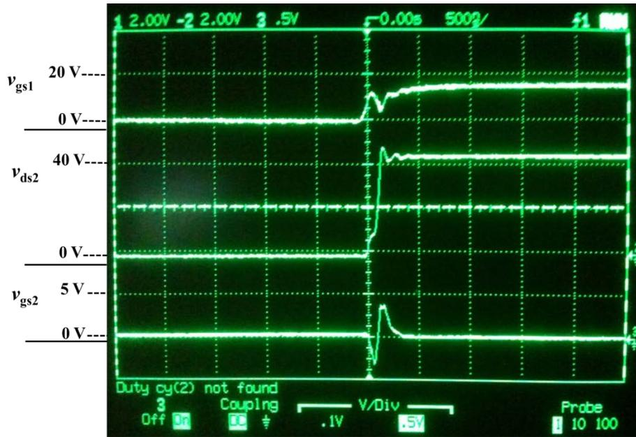
**Figure 26.** Experimental waveforms after  $C_{gd2}$  is raised to 1.25 nF. 10:1 testing probes were used for measurement, while the scope measurement is set to 1:1.
