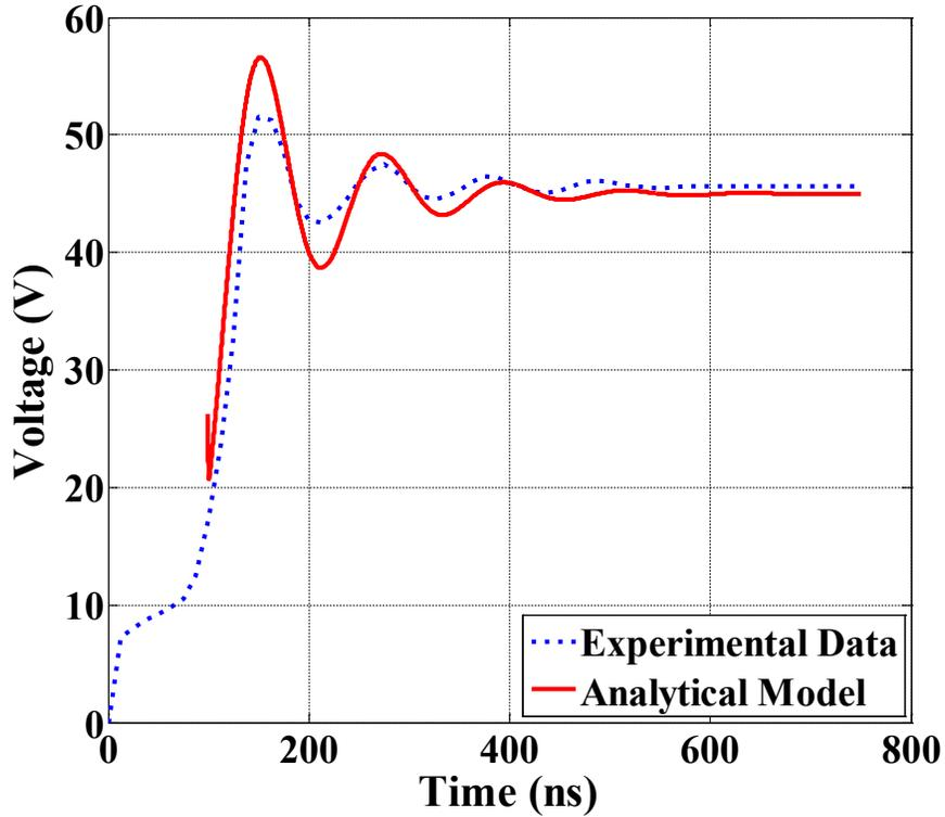
Figure 19. Step response for  $v_{ds2}$  compared with experimental  $v_{ds2}$ .
