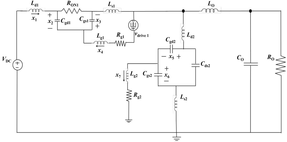
**Figure 21.** Definition of state variables in equivalent circuit of synchronous buck converter
