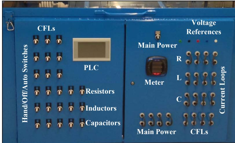
**Figure 61.** Detailed view of the front control panel.
