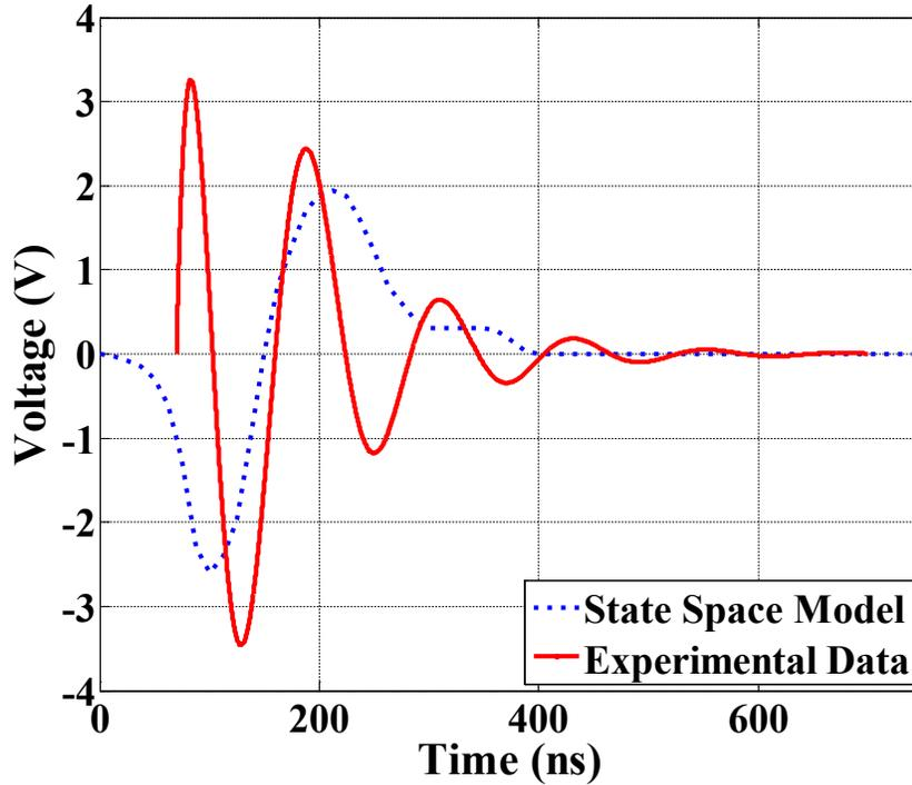
**Figure 20.** Step response for  $v_{gs2}$  compared with experimental  $v_{gs2}$
