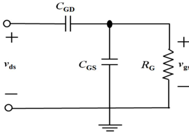
**Figure 6.** First order circuit model for transistor in off-state [19]
