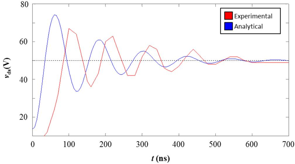
**Figure 9.** Analytical and experimental step response for  $v_{ds}$
