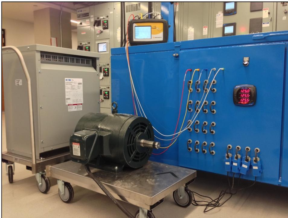
**Figure 64.** Experimental setup for testing and validation of motor loads.
