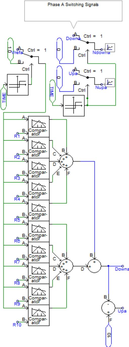
**Figure 54:** Calculation of the number of ON cells in the upper and lower arms
