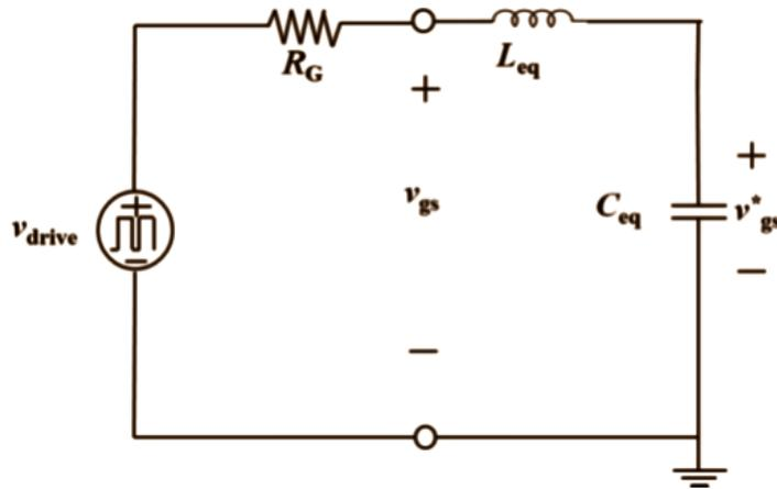
**Figure 4:** Gate charging circuit
