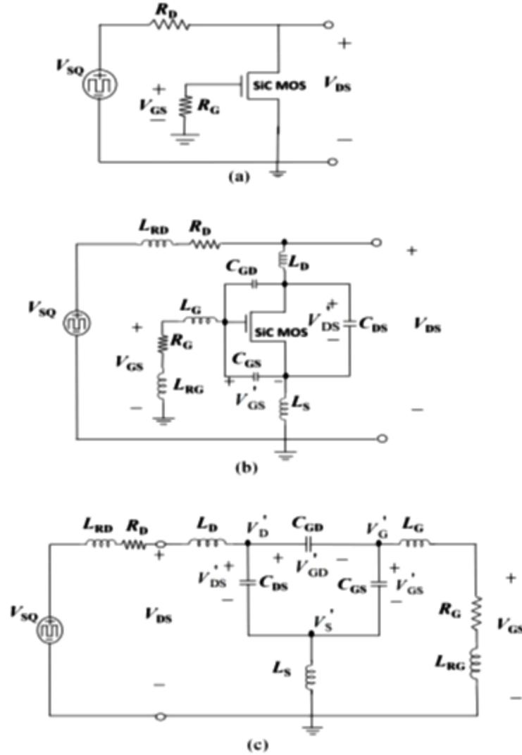
**Figure 7.** (a) High  $dv/dt$  test circuit. (b) Test circuit including parasitic components. (c) Equivalent test circuit with SiC MOSFET in off state.
