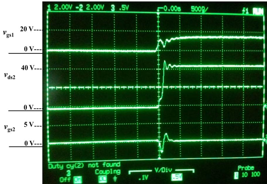
**Figure 13.** Experimental waveforms for false turn-on. 10:1 testing probes were used for measurement, while the scope measurement is set to 1:1.
