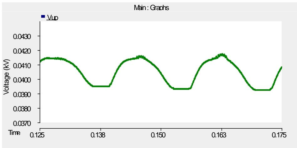
**Figure 57.** Balanced voltage in upper arm capacitor under balancing control
