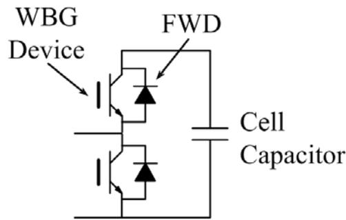
**Figure 48.** Half-bridge submodule topology for MMC inverter
