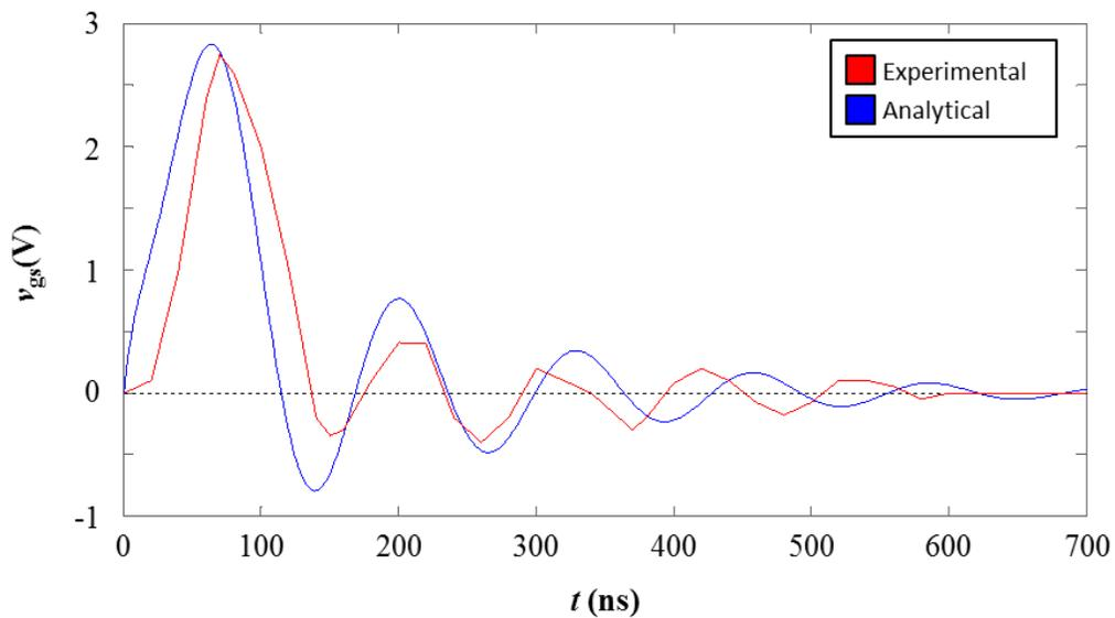
**Figure 8.** Analytical and experimental step response for  $v_{gs}$
