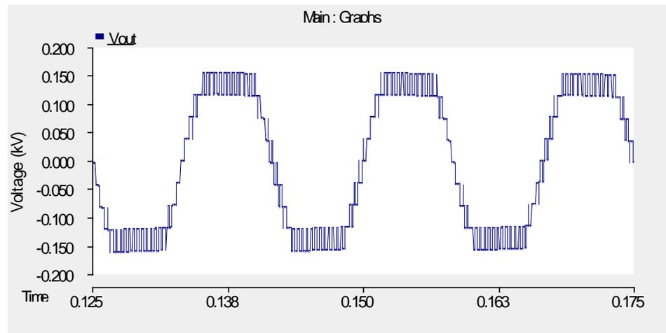
**Figure 58.** Voltage output from single phase, 10 cell, MMC inverter
