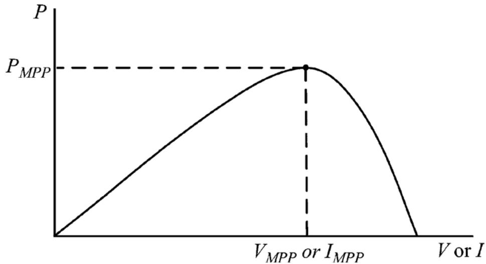
**Figure 28.** Power versus voltage or current for PV panels
