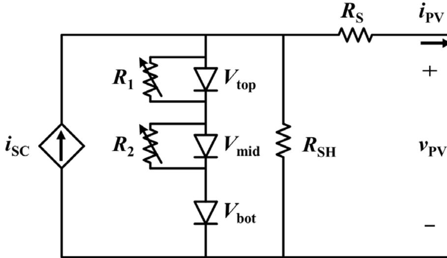
**Figure 30.** Piecewise linear PV module model based on diode turn-on [35]
