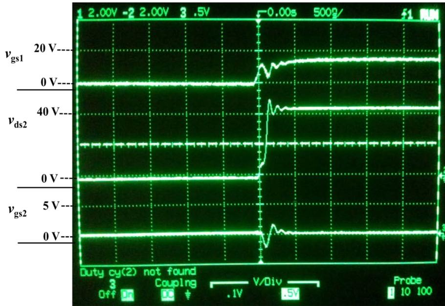
**Figure 27.** Experimental waveforms after  $C_{gs2}$  is raised to 20.75 nF. 10:1 testing probes were used for measurement, while the scope measurement is set to 1:1.
