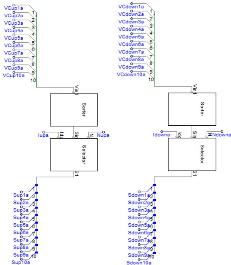
**Figure 55:** Sorting and Selection Modules for the Upper and Lower Arms of Phase A
