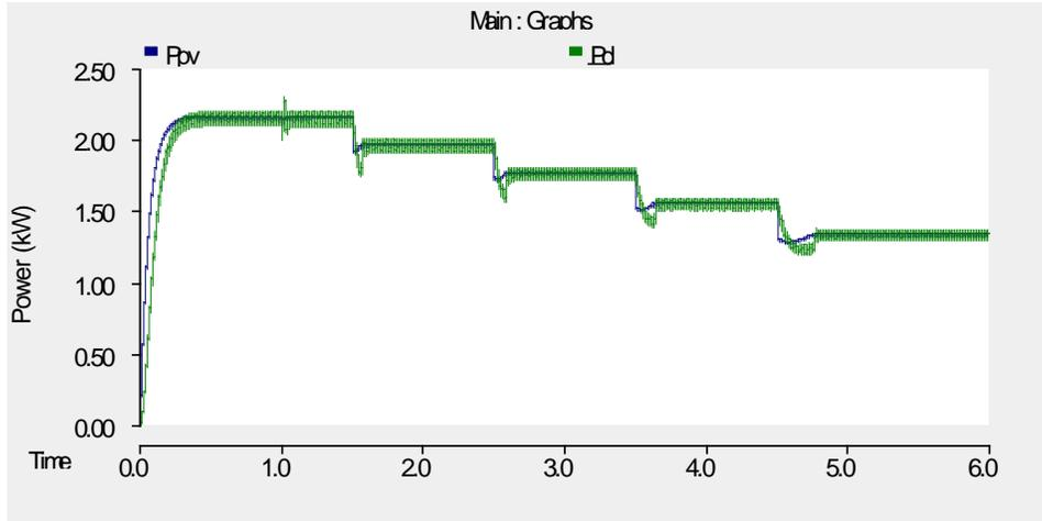
**Figure 43.** Test Condition II: input and output power waveforms
