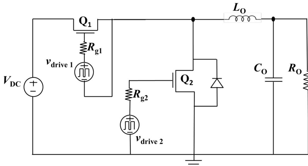
**Figure 12.** Synchronous buck converter
