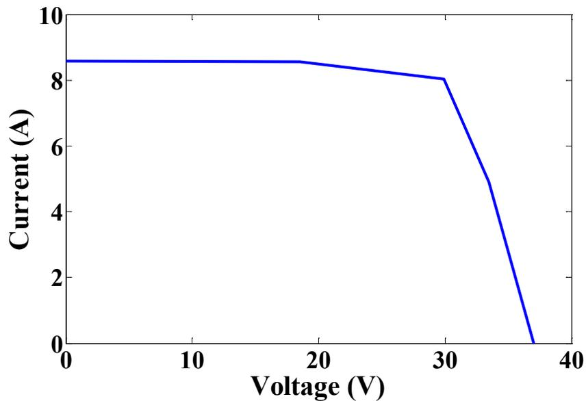
**Figure 33.** V-I curve for CanadianSolar CS6P-240P generated by the piecewise linear model
