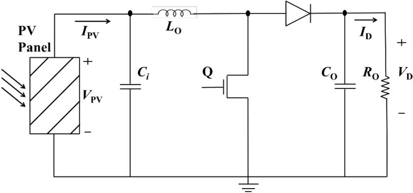
**Figure 29.** PV connected DC-DC boost converter system for MPPT
