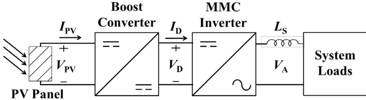
**Figure 1.** Complete PV system. From left to right: PV panel model, boost converter, MMC inverter, and dynamic system loads
