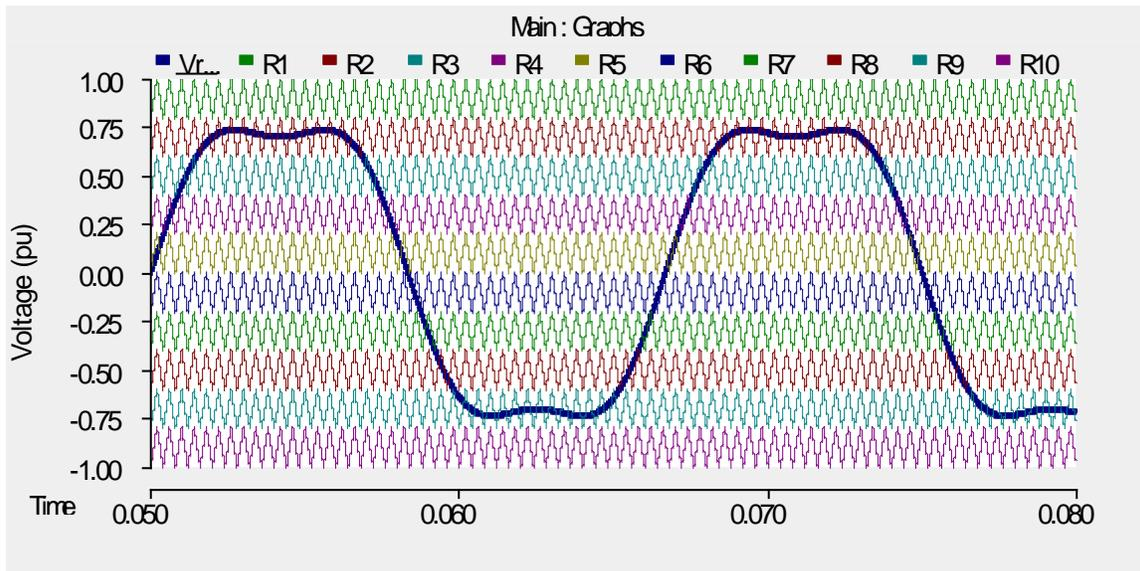
**Figure 53:** Reference and carrier waveforms for switching algorithm
