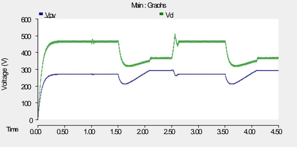
**Figure 46.** Test Condition III: input and output voltage waveforms
