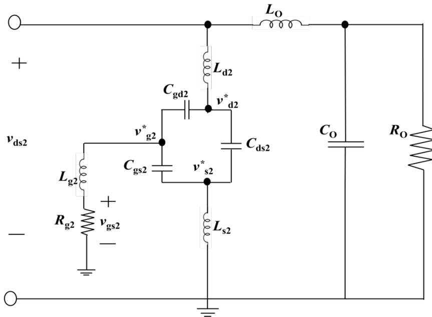
**Figure 17.** Equivalent circuit for  $Z_{eq}$  of Figure 16 with node voltages indicated for  $Q_2$
