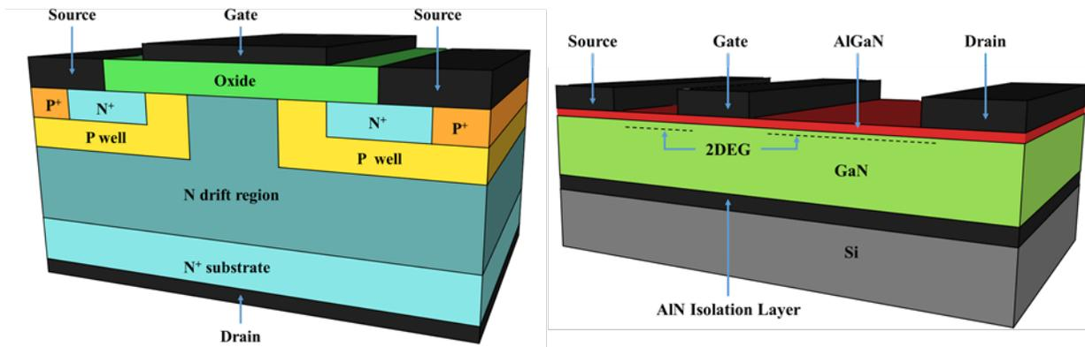
**Figure 2.** Transistor structures. Left: SiC MOSFET, Right: GaN HEMT
