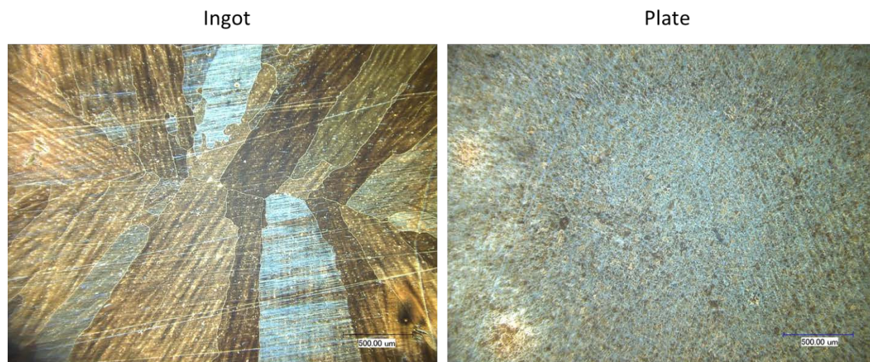
Figure 85: Microstructure of batches FeNiCr alloy that came from an ingot and a plate (same magnification)
