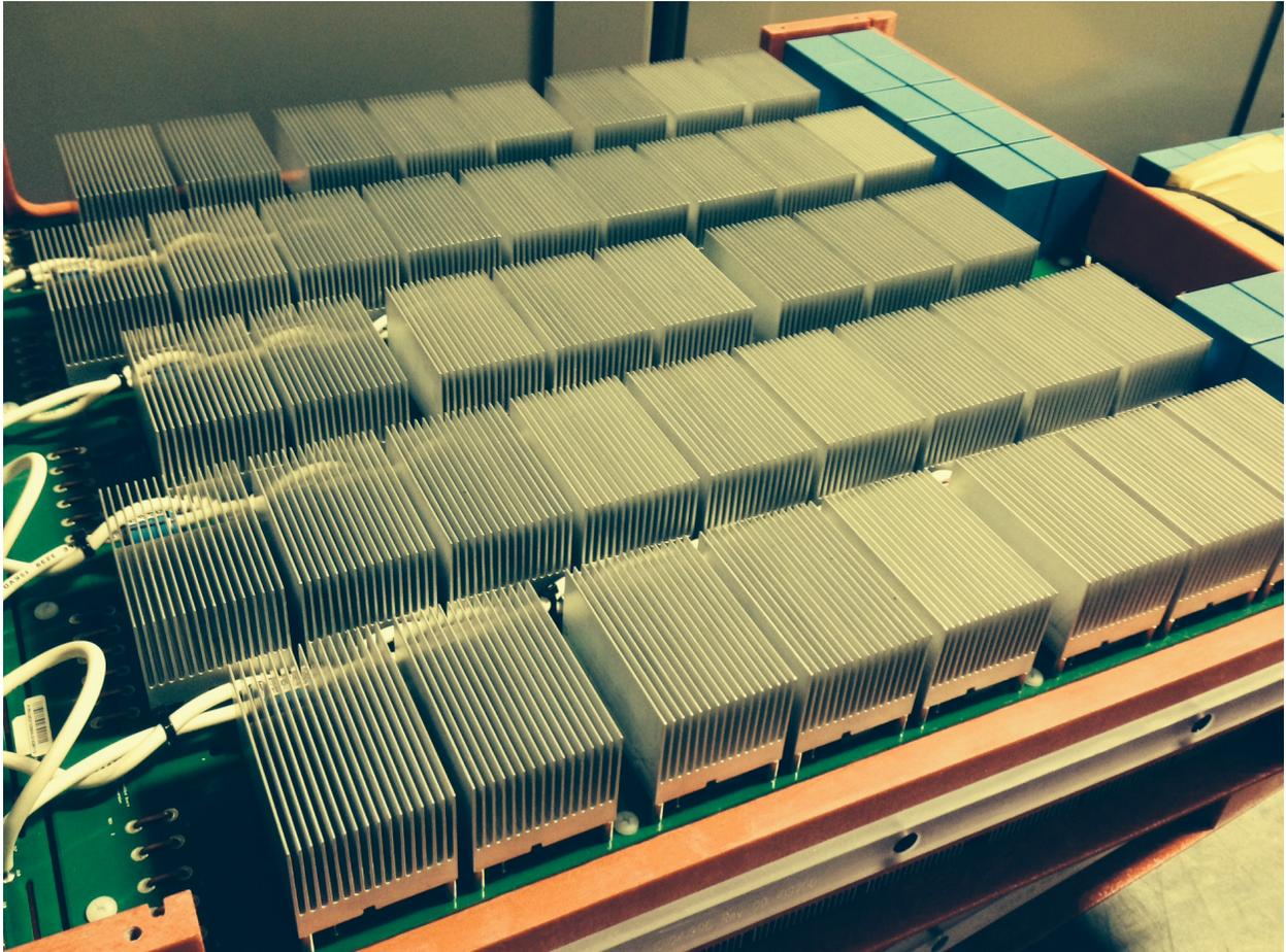
Figure 12.2: Sub-circuit 1 PCB shown with heat sinks.
