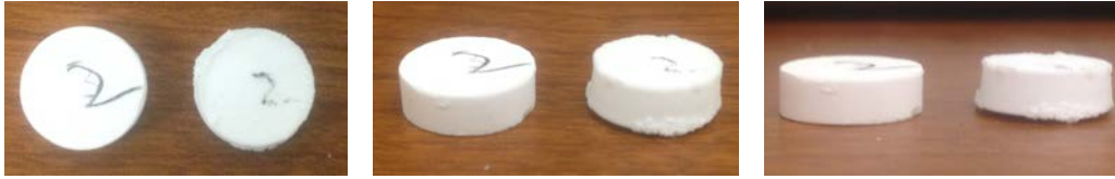
Figure 20: Pellets sintered at 1300°C (Right) and 1250°C (Left) from different direction
