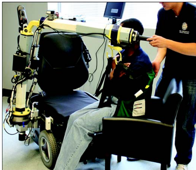
Figure 1. Strong Arm assists with clinician transferring person in sling attached to Strong Arm from electrical powered wheelchair to other surfaces.
