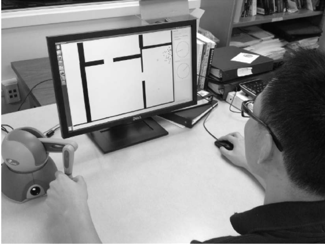
Figure 2. Participants used an Omni Phantom device (left) and mouse to influence the swarm and control the interface
