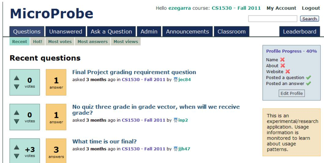
**Figure 3.** Main User Interface of MicroProbe. The tabs at the top allow users to navigate to different functionality. Gamification concepts such as points and leaderboards were added to motivate participation.
