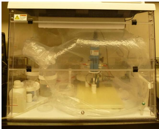
**Figure 3-6.** Image of electrode rotator in a Ar-filled polyethylene glove bag. The bag was accommodated in a class 100 laminar flow hood.
