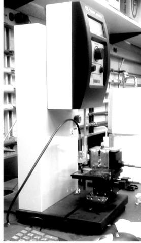
Figure 5.1: Micromechanical force microscope: Brookfield texture analyzer casing, stainless-steel retractible cantilever, optical displacement sensor.
