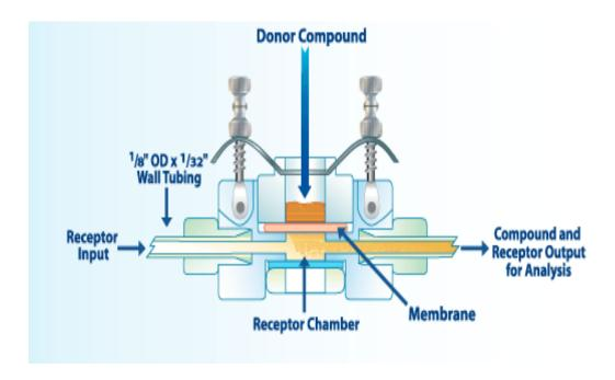
Figure 26 In-line cell for tissue permeability study.
