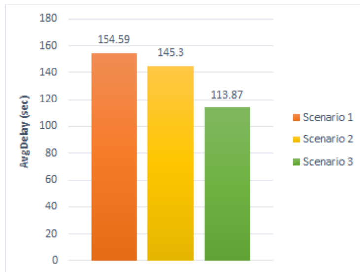
Figure 9. Average delay per vehicle in the Baum-Centre Corridor network during PM peak
