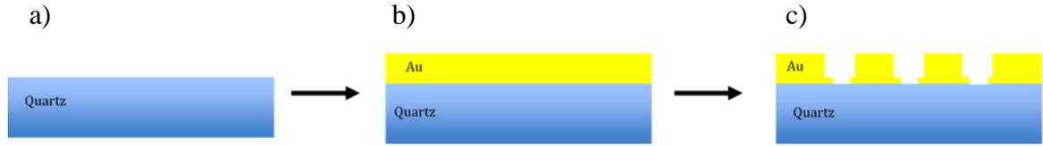
**Figure 2.2** Schematic of FIB milling routine employed for fabricating the nanoledge structure. a) Cleaning the substrates; b) Thin metal film deposition; and c) FIB milling of the targeted nanoledge structure.
