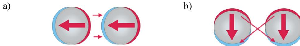
**Figure 1.6** Nanoparticle coupling under a longitudinal restoring force (a) shifts the resonance to lower frequency and nanoparticle coupling under a transverse polarization (b) increases the restoring force through coupling to neighbors shifting the resonance to higher frequency.
