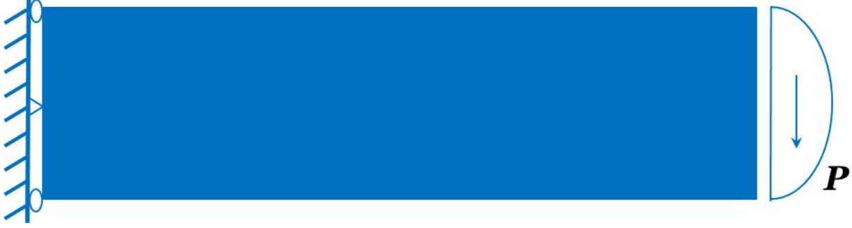
Figure 5.8: A 2D beam commonly employed in solid mechanics to test the convergence of FEM
